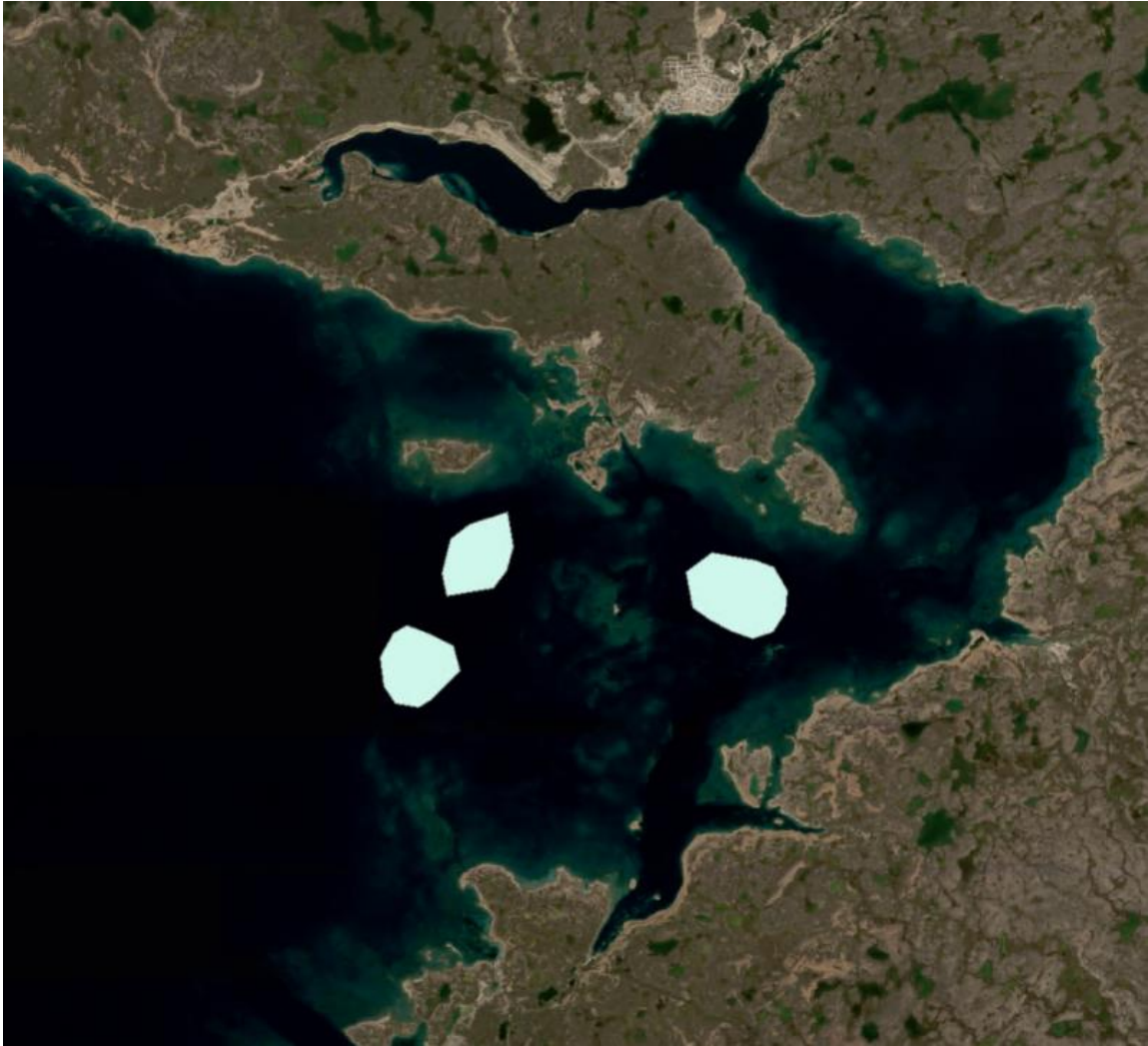
Figure 20 – Initial multispectral GeoTIFF file made with the coastal, blue, green, red, and NIR bands, as well as a shapefile with varying amounts of sun glint.
