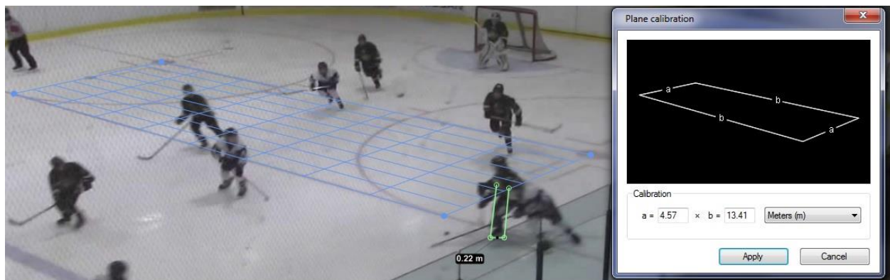
Figure 5. Perspective grid calibration and distance travelled shown at 5 frames prior to an elbow to head impact event.
