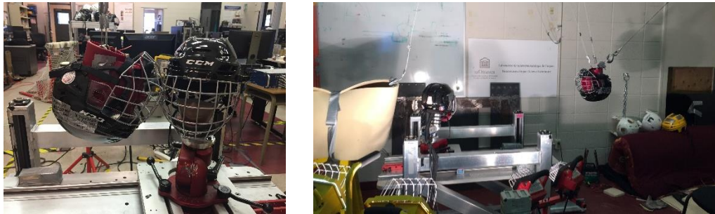
Figure 11. Head to head NOCSAE striker attached to the swinging pendulum impactor system.
