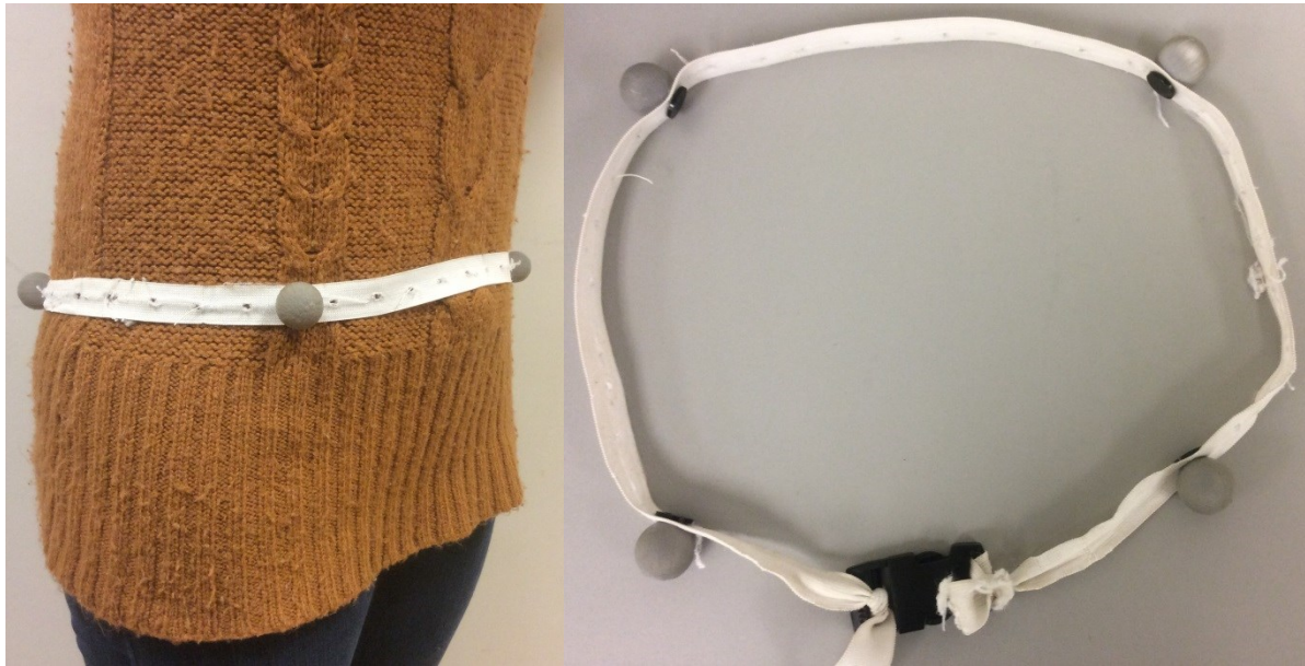
Figure 1. Belt used for the external focus condition. The lightweight elastic belt is outfitted with two markers on the ventral side and two on the dorsal side, which are aligned with the anterior and posterior superior iliac spines, respectively.
