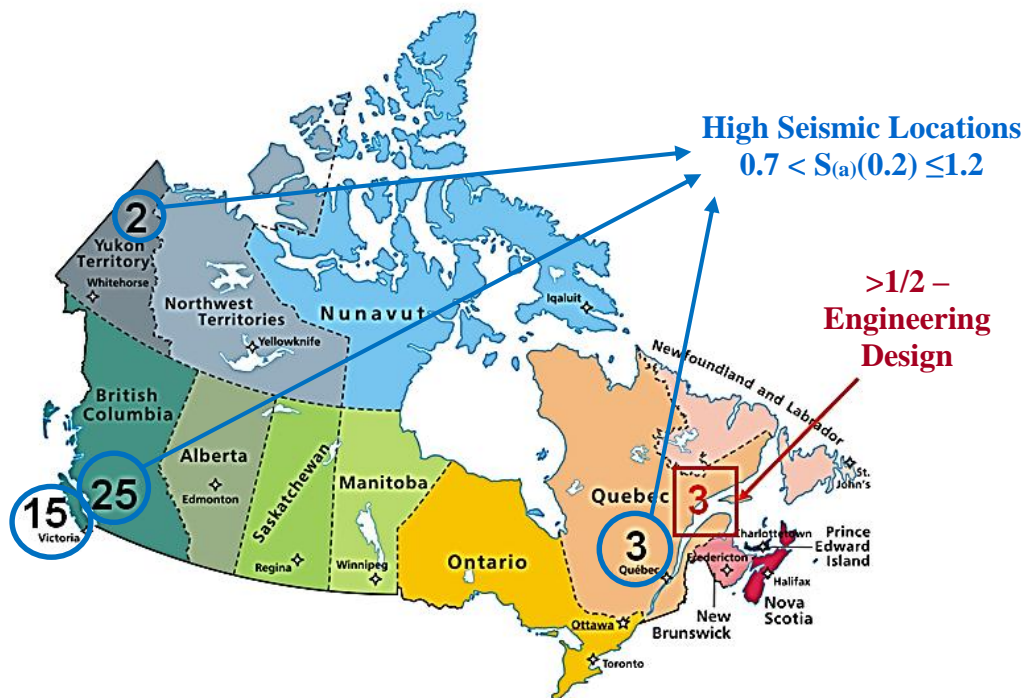
Figure 2-11: The Impact of the New Categorization, Proposed in Part 9 of NBCC 2010, Across Canada, Due to Earthquake (NRCC, 2011; Taraschuk, 2011)
