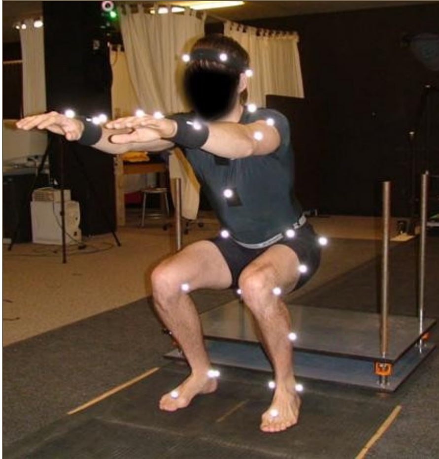
Figure 3.7: Maximal squat depth analysis. Participants performed dynamic squats with both feet on AMTI force plates with retro-reflective marking anatomical positions and VICON motion capture cameras recording kinematics. Reproduced with permission of Springer from Lamontagne, et al., 2009.
