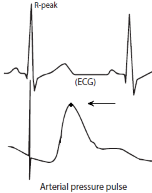
Figure 2.4: Pressure peak identifying approach based on simultaneously recorded ECG and oscillometric signal. The identified peak in the pressure pulse is shown with a dot (Adapted with permission from Forouzanfar, 2014).
