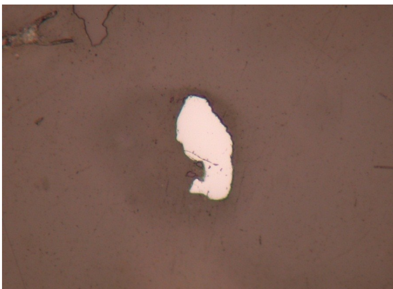
Figure A.45. Photomicrograph of magnetite under plane polarized reflected light in specimen CA-76 (PPOL, FOV = 0.55 mm).
