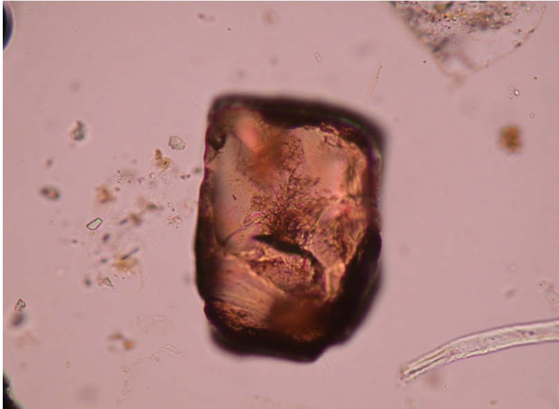
Figure A.12. Photomicrograph of garnet grain in specimen BA-45 (PPOL, FOV = 0.55 mm).
