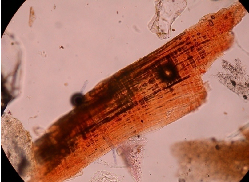
Figure A.9. Photomicrograph of hardwood cellulose in house dust of specimen BA – 37 (PPOL, FOV = 0.55 mm).
