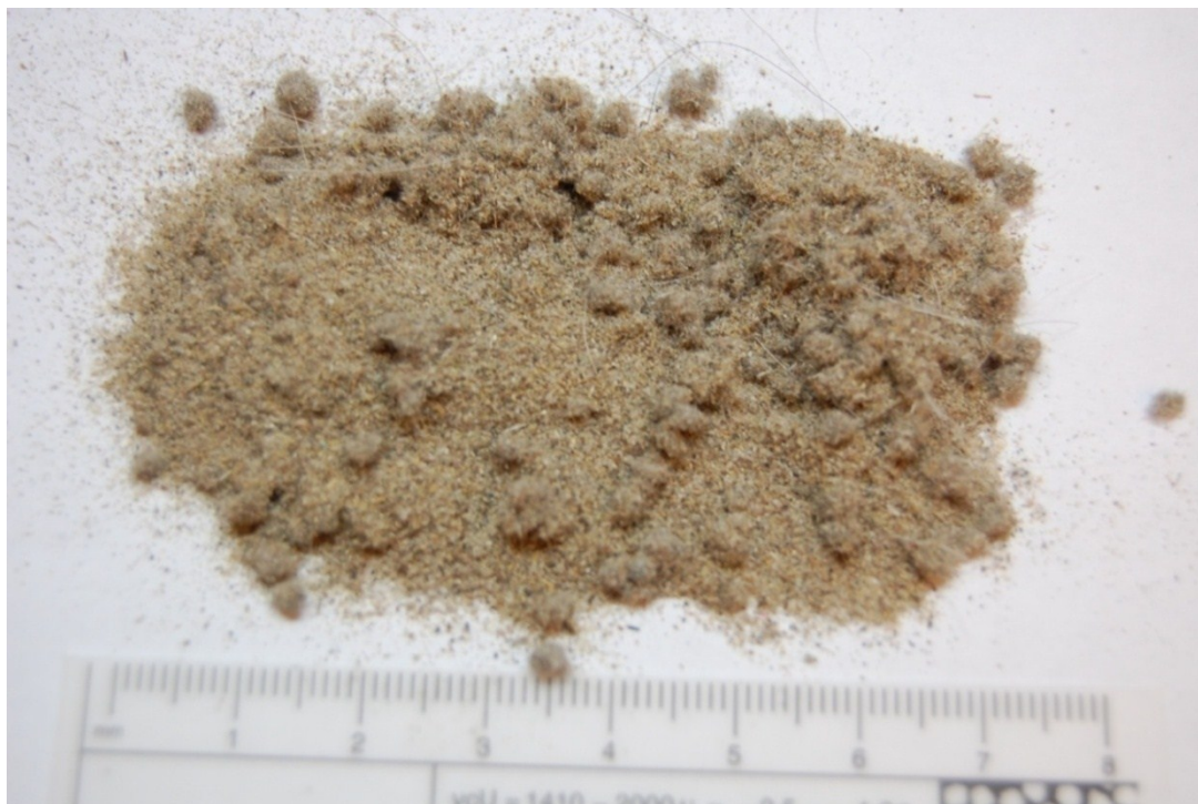
Figure 3.1 Representative example of vacuumed specimen of house dust (80 - 300 \mu\text{m} ).
