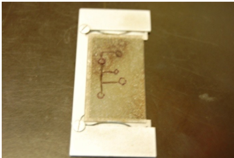
Figure 3.2 Polished thin section of house dust (30 \mu\text{m} ) in microscopic stage holder.
