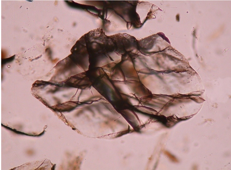
Figure A.6. Photomicrograph of perthitic feldspar grain (PPOL, FOV = 0.55 mm).
