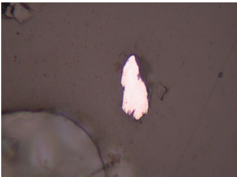
Figure A.21. Metallic particle/copper wire under plane polarized reflected light in specimen BA - 54 (PPOL, FOV = 0.55 mm). (The grains are opaque under plane polars).
