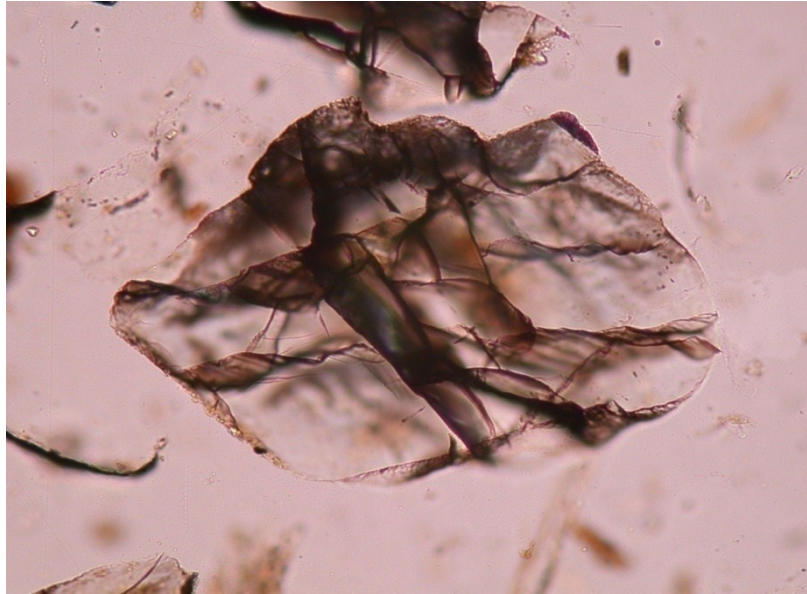
Figure 4.3. Photomicrograph of a turbid feldspar grain (PPOL, FOV = 0.55 mm).
