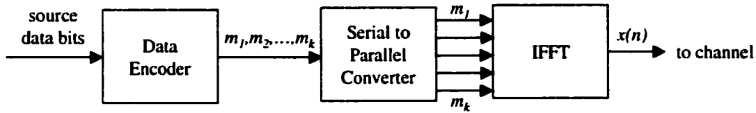
Figure 3-3: OFDM Modulator.
