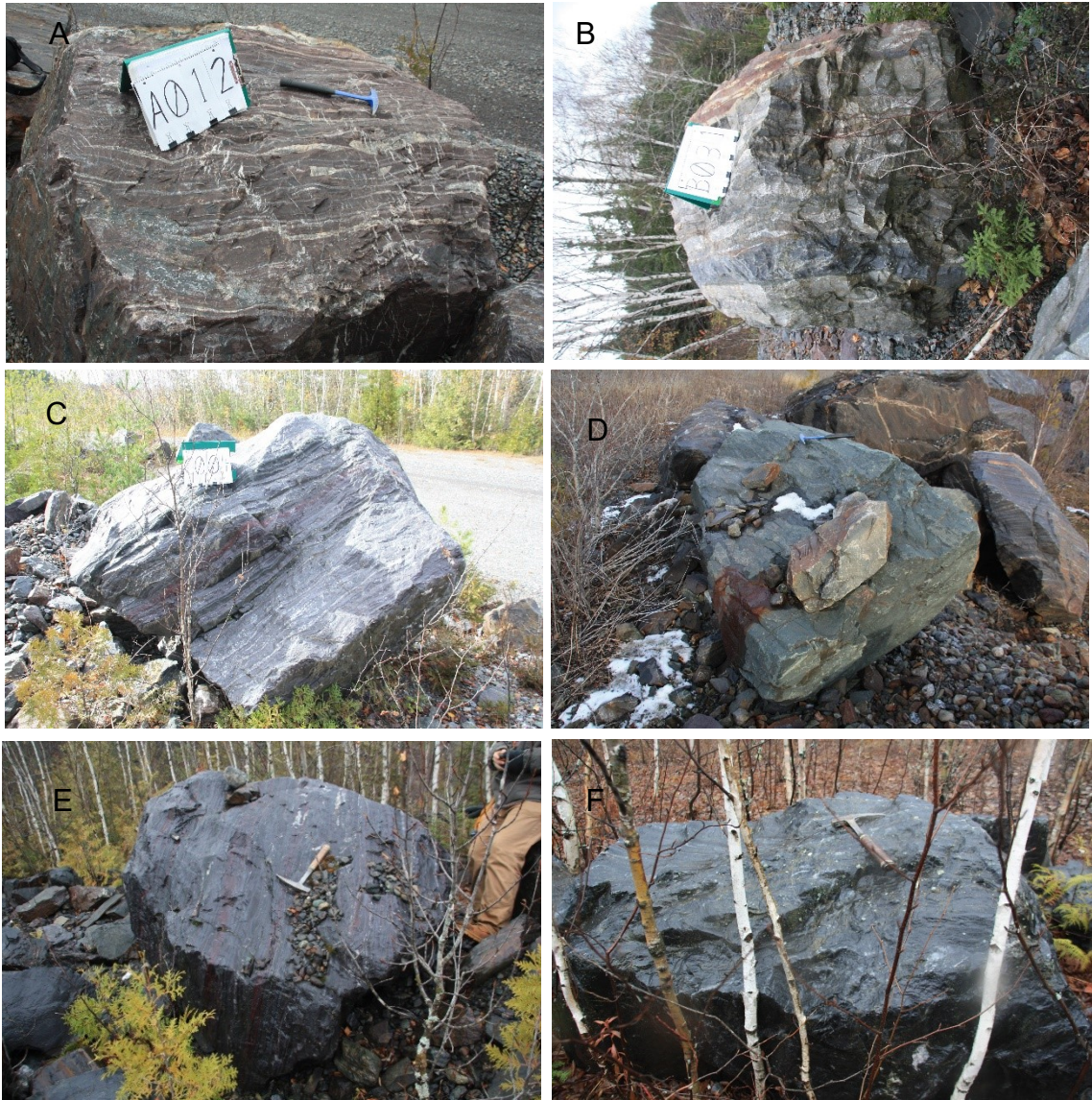
Figure 5.4 Field photographs of representative large ore blocks from the Sherman Mine pits. A) Block A013: black chert-dominated BIF. B) Block B031: white chert-dominated BIF. C) Block C004: magnetite and jasper BIF from the C-series. D) Block D001: chlorite-rich BIF. E) Block E004: magnetite and jasper BIF from the E-series. F) Block F021: mixed chert and chlorite BIF.
