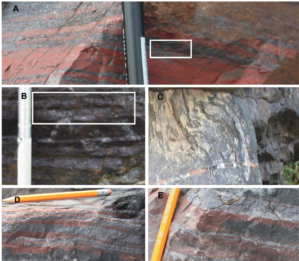
Figure 6.3 Field photographs of different layer Types of the Temagami BIF. A) Magnetite and jasper beds in an ore block from the southern pit of the Sherman Mine. The magnetite bands contain ~1mm jasper clasts (visible in the white box). B) Magnetite and black chert beds in a block from the northern pit of the Sherman Mine. Magnetite beds commonly include many white chert microbands (visible in the white box). C) Example of chlorite and chert beds with minor folding in the Highway 11 outcrop. D) Jasper, magnetite and black chert layers in a block from the southern pit of the Sherman Mine. E) Photograph showing black chert “encroaching” on an original jasper layer.
