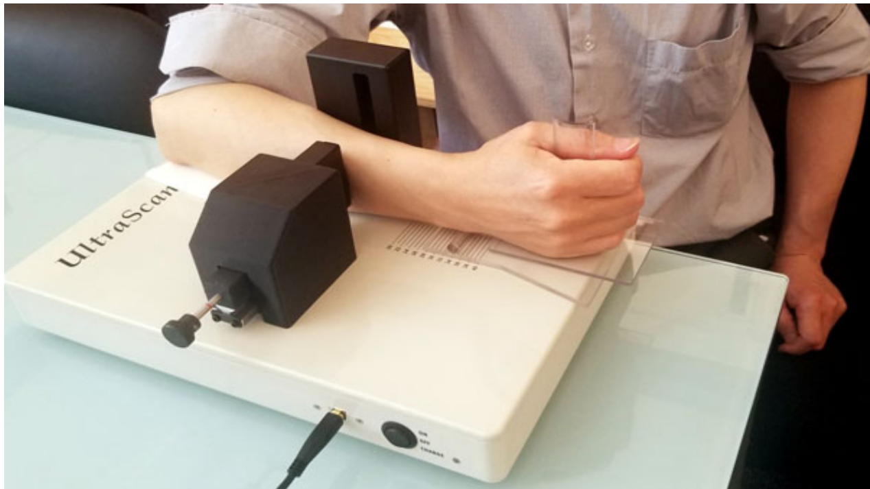
Appendix 5. Participant's positioning for UltraScan650™ measurement of the 1/3 rd distal radius. Image taken from Stein et al.
