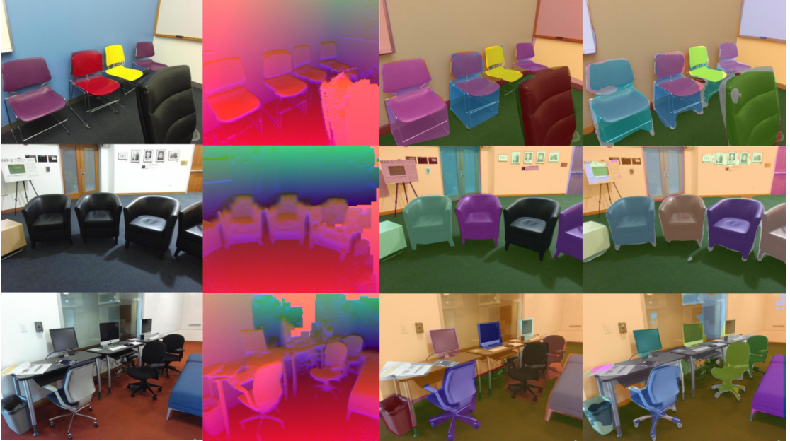
Figure 5.12: Predicted masks from the Depth-Aware Panoptic model on the SUN RGBD dataset overlaid over the RGB image. From left to right: RGB Image, HHA Image, Ground truth panoptic mask overlay, Predicted panoptic mask overlay.
