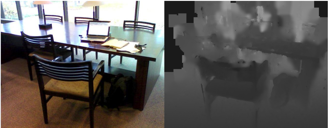
Figure 4.3: Left: An RGB image, Right: A very noisy depth image. Images taken from the SUN RGBD dataset [8].
