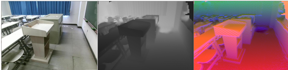
Figure 2.5: An example HHA image obtained from an RGBD image from the SUN RGBD dataset [8]. Left: RGB Image, Middle: Depth Image, Right: HHA Image.
