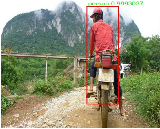
Figure 2.9: The output from an object detection model input with an image from the MS-COCO dataset [23], showing a bounding box, a confidence score, and a class label.
