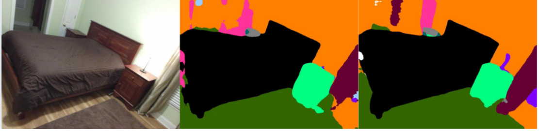
Figure 5.9: Comparing the qualitative output of the RGB DeepLabv3 baseline to the Proposed DeepLabv3 f_{Res} model on an image from the SUN RGBD dataset. Left: RGB Image, Middle: RGB DeepLabv3 output, Right: Proposed DeepLabv3 f_{Res} output.
