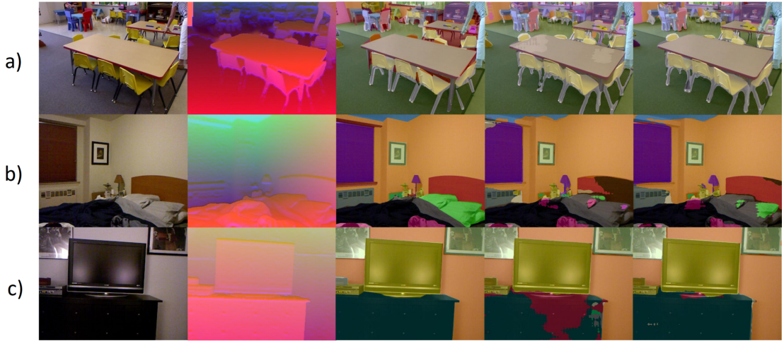
Figure 5.7: A visual comparison of the semantic segmentation masks predicted by the depth-aware DeepLabv3 f_{LC} model compared to the RGB baseline on images from the NYUDv2 dataset. Segmentation masks are overlaid over the original image. From left to right: RGB image, HHA image, ground truth segmentation mask, RGB DeepLabv3 output, DeepLabv3 f_{LC} output.
