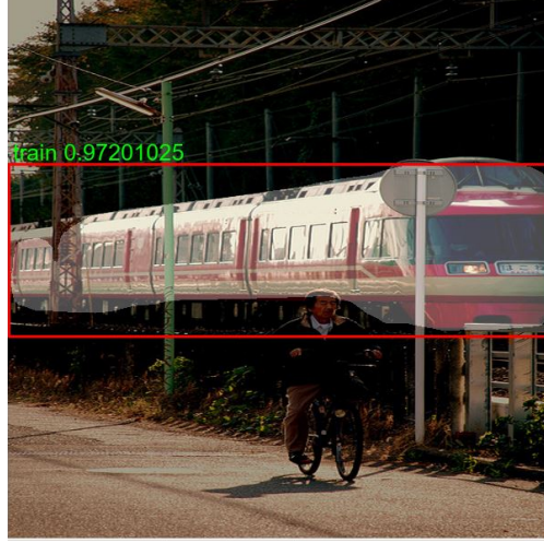
Figure 2.11: The output of an instance segmentation model input with an image from the Pascal VOC 2012 dataset [30] consisting of a bounding box, confidence score, class label, and an instance mask overlaid in white over the original color image.
