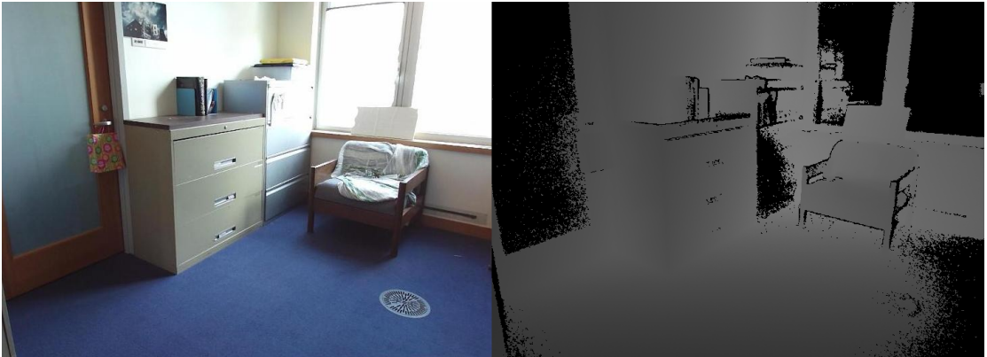
Figure 4.1: Observing noise patterns in a depth image from the SUN RGBD dataset [8].
