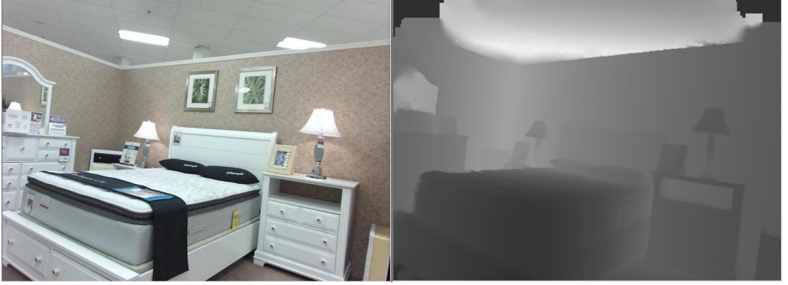
Figure 2.1: An RGBD image obtained from the SUN RGBD dataset [8] with the Kinect v2 depth camera.
