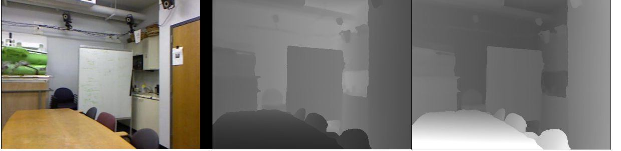
Figure 2.2: An example disparity image from the SUN RGBD Dataset [8]. Left: RGB Image, Middle: Depth Image, Right: Disparity Image.
