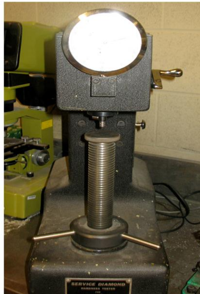
Figure 3-10: Rockwell tester used for determining macro hardness.
