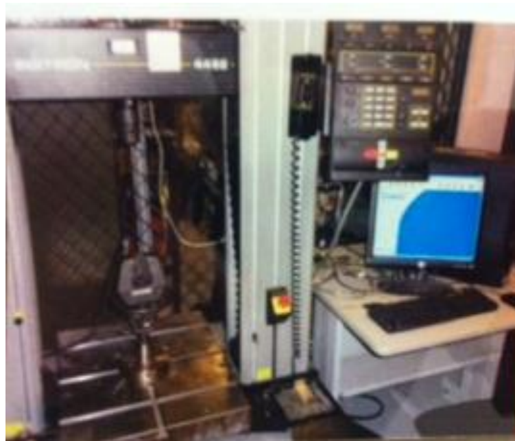
Figure 3-16: Computer controlled Instron universal testing machine used for the bend tests.
