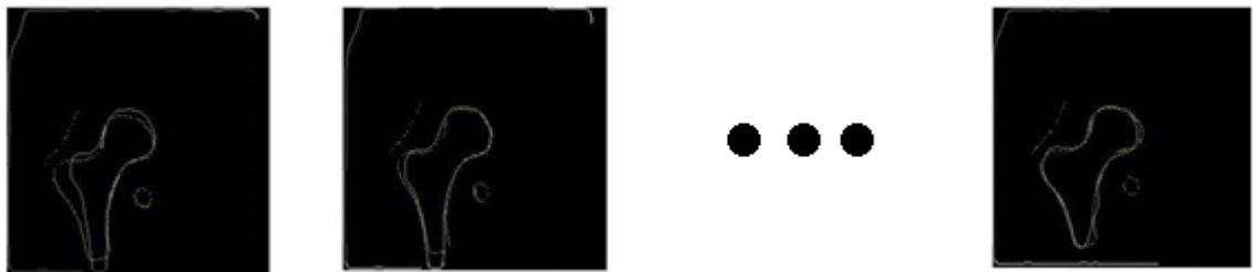
Figure 9: The global matching (level 0) of test images with all the training images. The edges shown are resulted by Canny edge detection and used for image matching.
