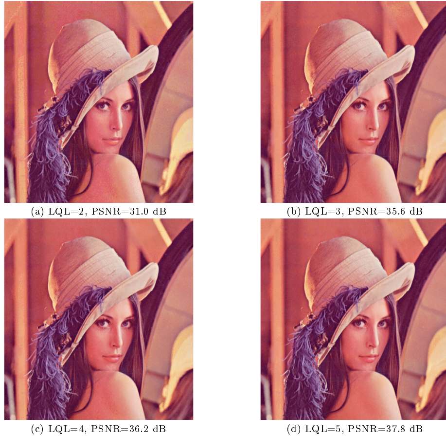
Figure 4.20: Reconstructed “Lena” by using different local quantization levels (LQLs).
