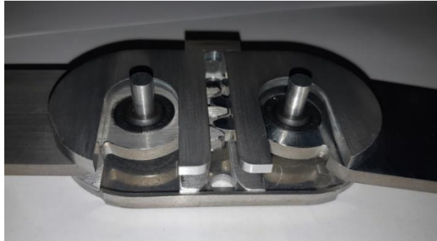
Figure 24: Interior view of the joint with faceplate, pad, machine screws, and wing nuts removed. The photo shows the press-fit spherical bearings in the uprights, the offloading plate, and the faceplate.
