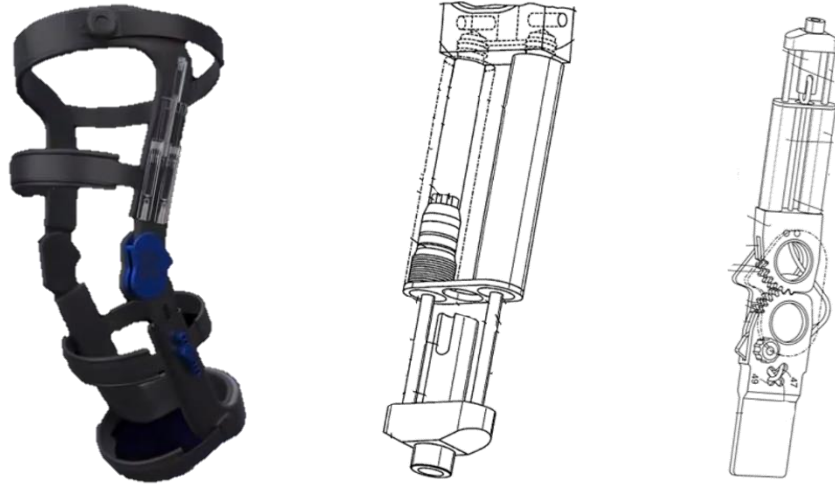
Figure 9: SpringLoadedTech Levitation knee orthosis commercial model (left) [85]. Patent images with labels removed for clarity in the center and right images show the spring cylinder system that controls the length of the cord attached to the lower upright [86]. Energy is stored in flexion and released to assist with extension.
