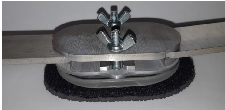
Figure 23: Manufactured prototype with a machine screw and wing nut. A plastic piece with fittings for the bolt heads with foam was added to demonstrate how it could be used against the knee joint.
