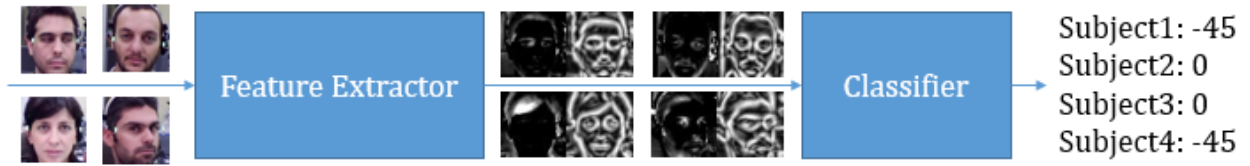
Figure 6. Head pose detector sub-components.
