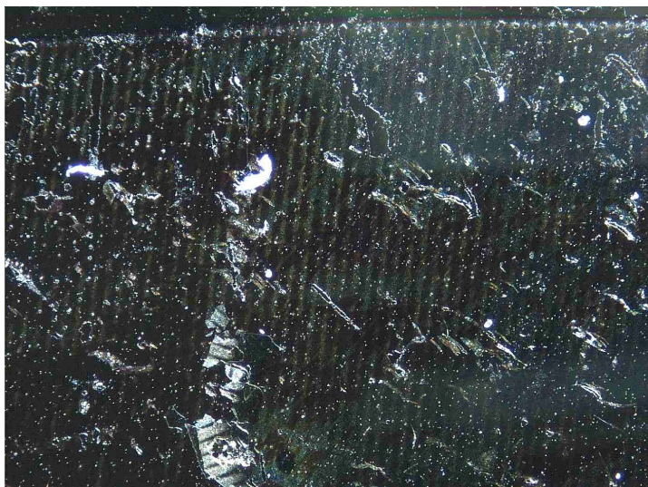
Figure 7.3 Optical microscope image of a DupXX film spin-coated from a 10% cyclohexanone solution onto a Si wafer, containing 1:1 AgOTf:I-2959 (10% w/p I-2959), exposed to 60 min irradiation (UVA, 6 lamps) through an 18 \mu\text{m} linear pattern mask followed by 30 min PEB @ 100°C and 7 min development in basic developer solution.
