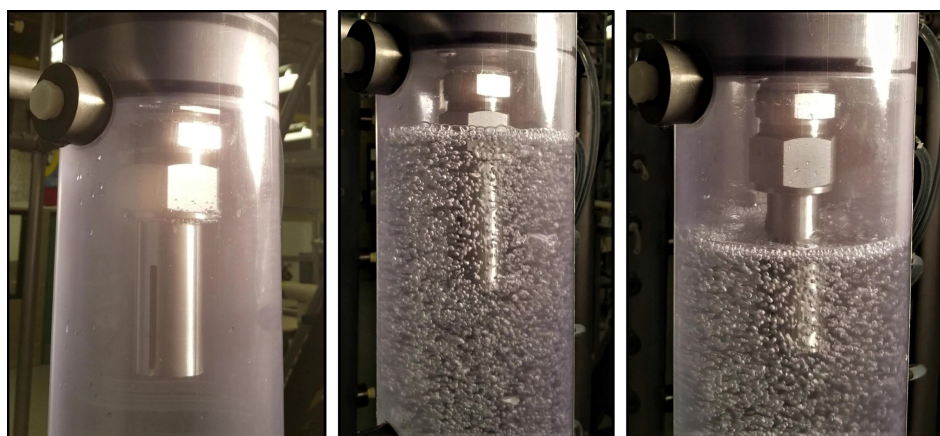
Figure 2.15: Plenum liquid level before and after switching the gas on ( U_L = 0.015 m/s, U_G = 0.01 m/s, air-water flow). Left most picture was taken with liquid flow but before the gas was introduced through a sintered pipe. The two pictures to the right were taken shortly afterwards and with gas flowing. The gas pocket formed due to bubble coalescence at the free surface grows over time until enough slit area is open to ensure both phases enter at the same pressure.
