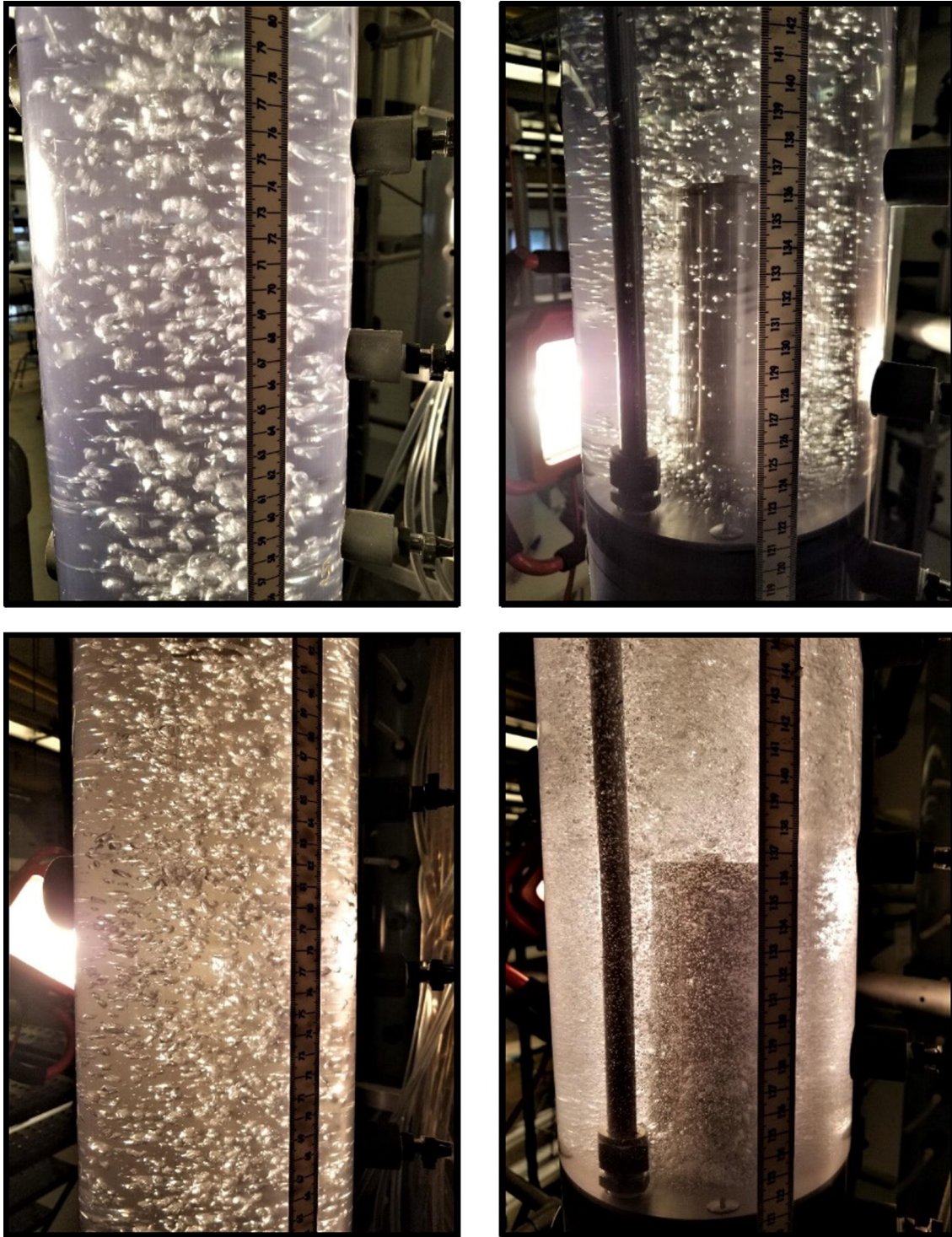
Figure 2.18: Bubble cap inlet and outlet conditions for air-water and air-water-ethanol flow, with perforated pipe gas sparger ( U_L = 0.015 m/s; U_G = 0.01 m/s). Top left: bubbles before entering the bubble cap, air-water flow; top right: bubbles emerging from the bubble cap, air-water flow; bottom left: bubbles before entering the bubble cap, air-water-ethanol flow; bottom right: bubbles emerging from the bubble cap, air-water-ethanol flow.
