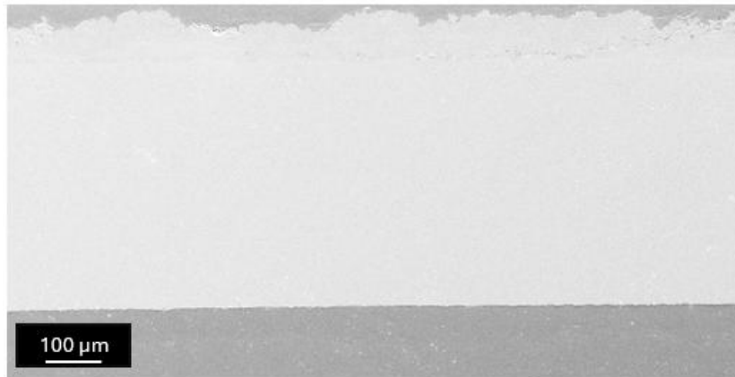
Figure 66: Cu coating on Cu substrate
