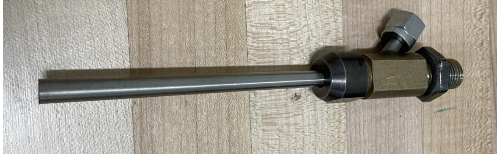
Figure 47: Steel nozzle assembly
