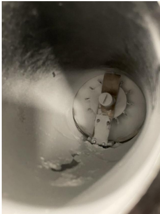
Figure 97: Nylon 6 powder sticking to the canister liner
