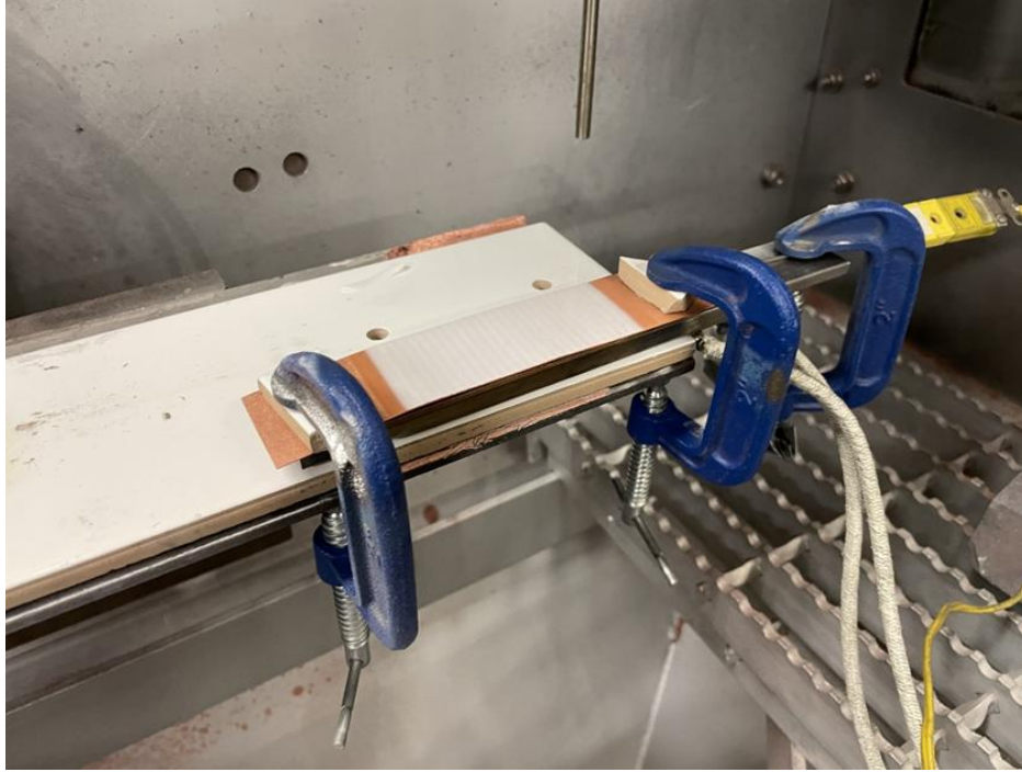
Figure 71: Successful coating of PFA onto Cu bond coat
