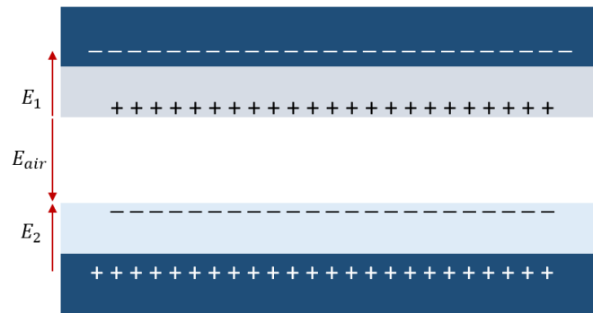
Figure 22: Electric fields in a VS-TENG
