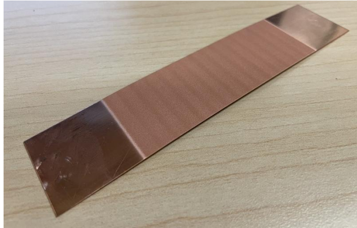
Figure 67: Cu coating on Cu substrate
