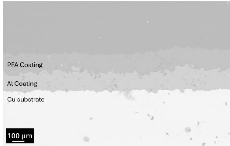
Figure 69: PFA on Al bond coat on Cu substrate
