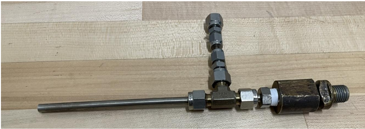
Figure 50: Straight section nozzle with injector attached
