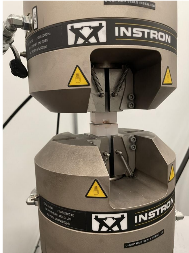
Figure 60: TENG mounted to Instron machine
