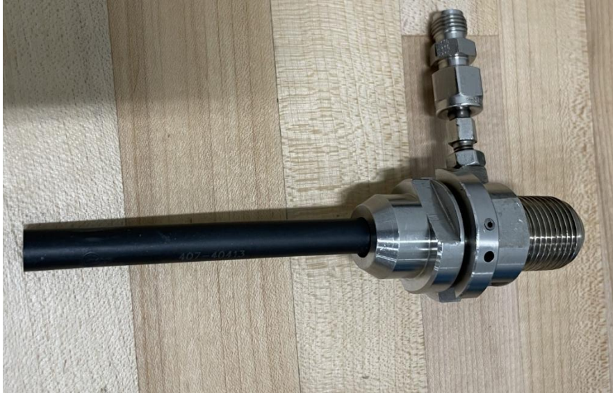
Figure 48: Polymer nozzle assembly
