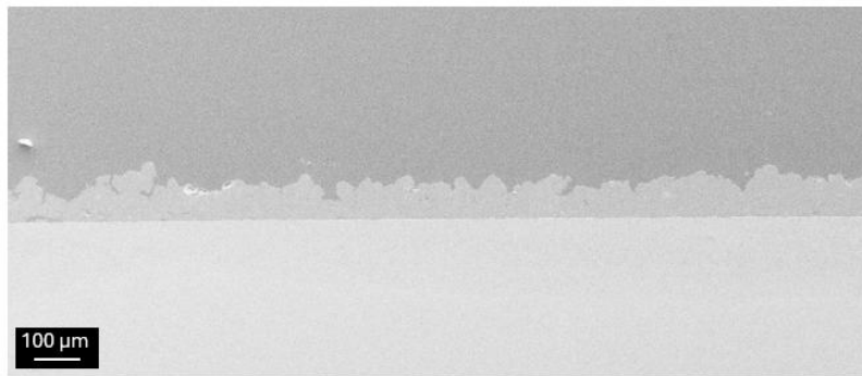
Figure 96: Al coating on Cu substrate after 6000 cycles
