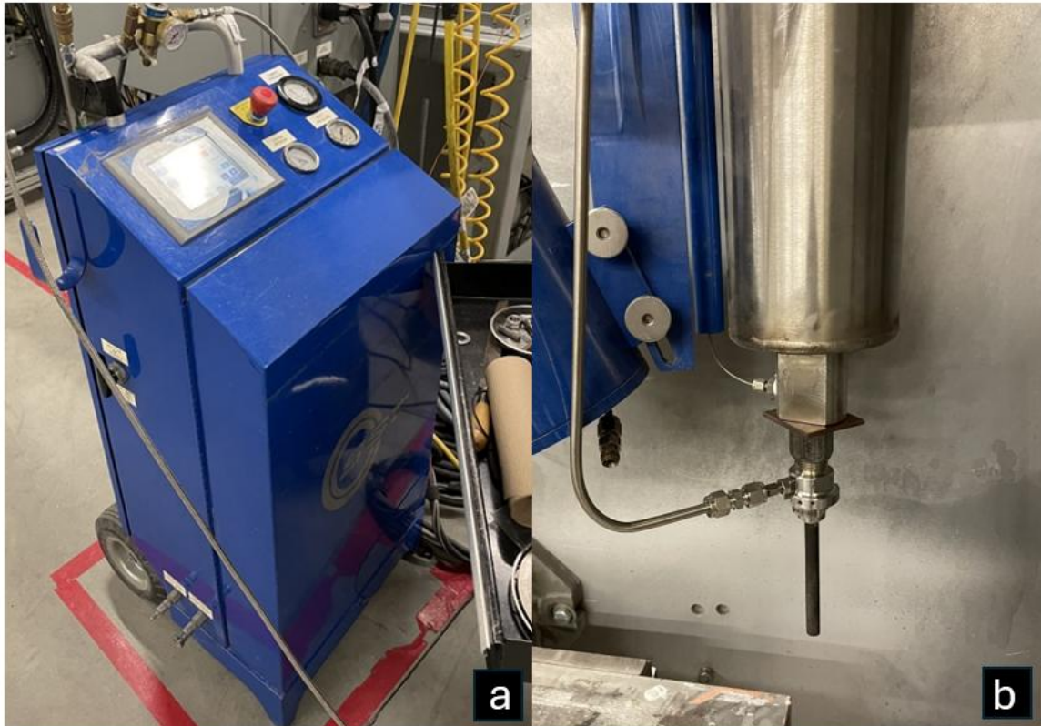
Figure 43: a) CS control unit b) Gas heater with nozzle attached
