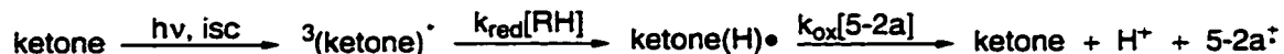
Scheme 5-9. Photoreduction of triplet-excited ketones by hydrogen donors (RH) and subsequent oxidation of the ketyl radicals by 5-2a .
