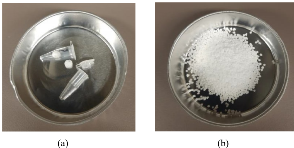
Fig. 4-1. 5 mm polyethylene particle used in the first approach (a); 1.2 mm polyethylene particle used in the second approach (b).
