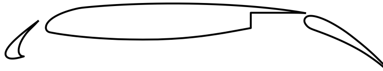
Figure 1.3: MDA 30P30N three-element airfoil
