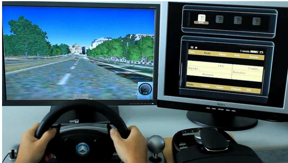
Figure 2.3: Prototypical implementation of an in-car-infotainment system
