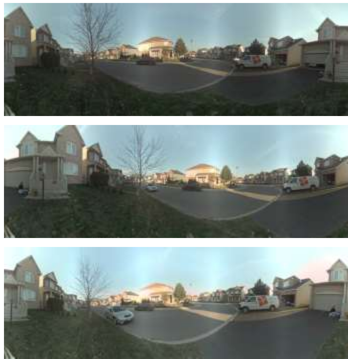
Figure 4.7 Cylindrical images captured at three positions with different exposures used as input for geometric calibration.
