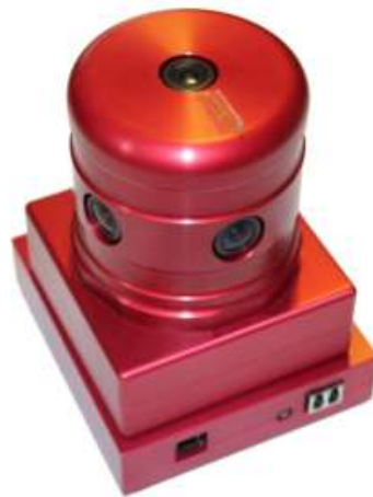
Figure A.1 Photograph of the Ladybug 2 camera system used for the image capture.
