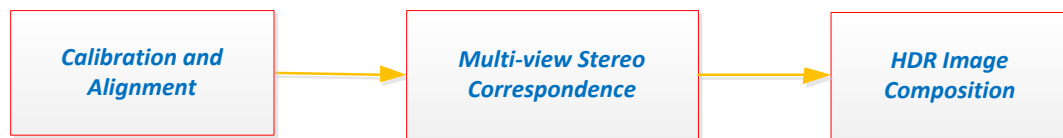
Figure 1.2 Pipeline of the multi-view omnidirectional HDR imaging
