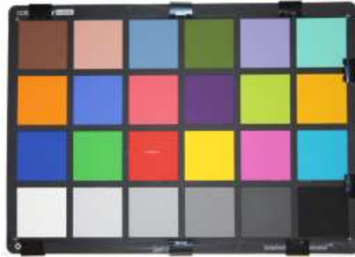
Figure 3.3 Photograph of the MacBeth ColorChecker test chart [94]. The bottom six gray patches from bright to dark are used for white balance and photometric calibration.
