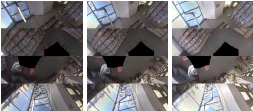
Figure 4.9 RD-map images with three different exposures. From left to right: low, medium and high exposures.
