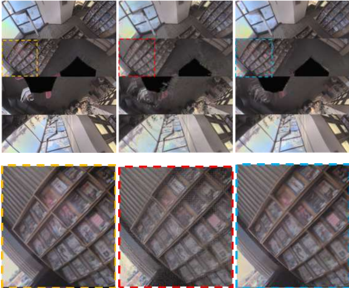
Figure 6.7 Comparison of tone mapped temporal HDR image (left) and spatiotemporal HDR images obtained using the disparity-based forward (middle) and backward (right) warping algorithms. Whole (top row) and partial (bottom row) images for Position #1.
