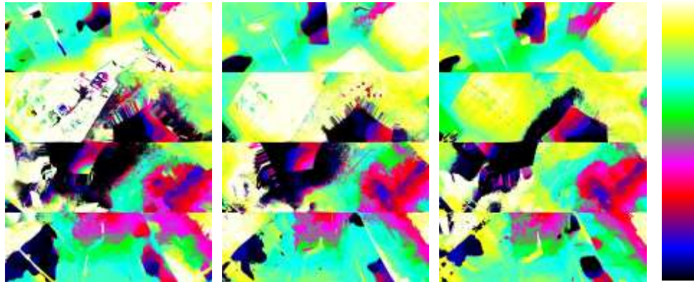
Figure 4.12 Disparity map derived using mutual information method. The color bar on the right indicates the minimum to the maximum disparity values upwards.
