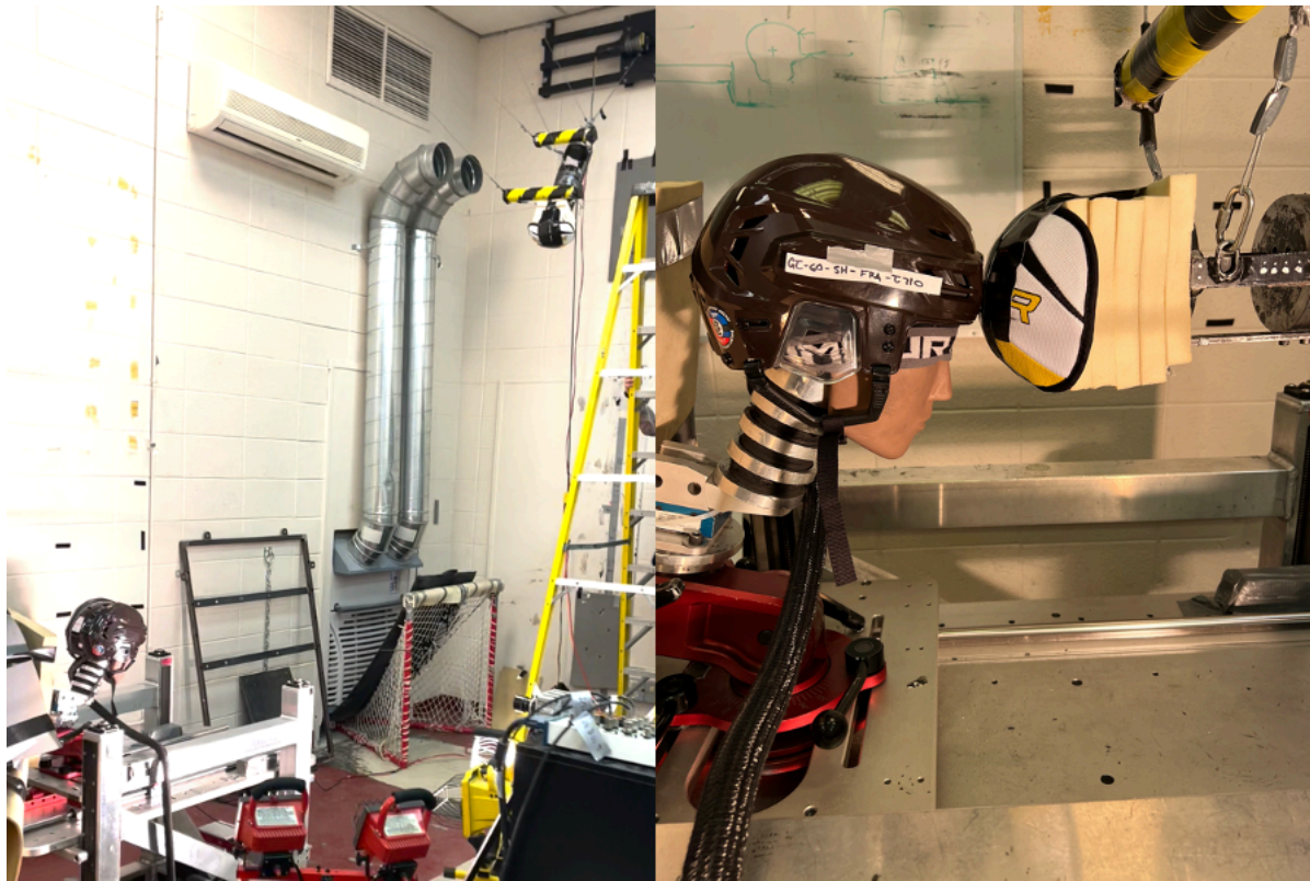
Figure 2. Pendulum drop rig set up.
