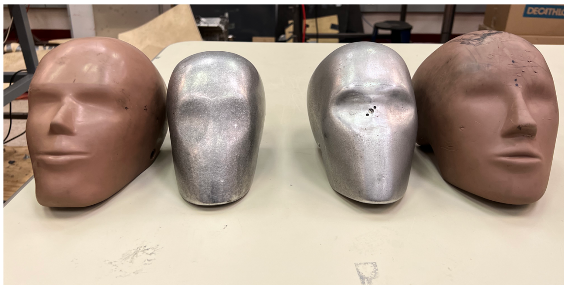
Figure 3. The Hybrid III 5 th percentile headform (left) and the Hybrid III 50 th percentile headform (right).
