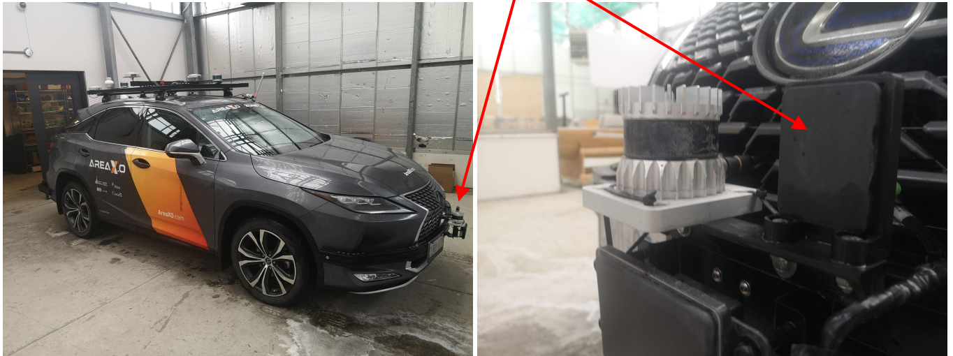
Figure 8.1: Instrumented vehicle with V-MD3 radar installed
