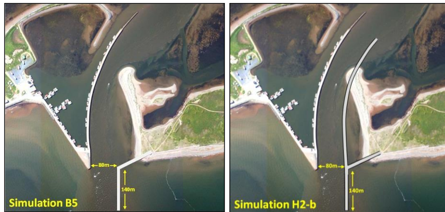
Figure 4.2 – Schematic of scenarios B5 and H2b; 2 of 17 scenarios modelled in the phase I study (from Logan, 2012).
