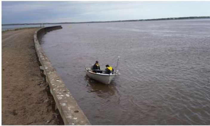
Figure 5.3 - Collecting ADCP data near the curved training wall (red transect).
