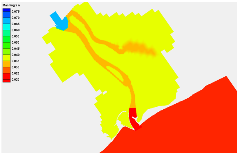
Figure 6.18 - Optimized map of Manning's coefficient values used in the current study.
