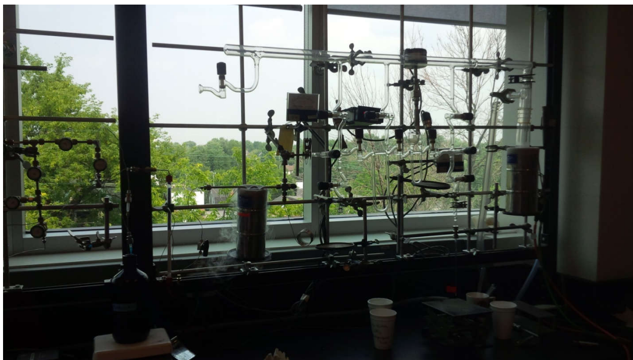
Figure 22. Set-up of the Ice-line extraction apparatus at the G.G. Hatch Stable Isotope Laboratory, University of Ottawa. The Ice-line was used for the extraction of CO 2-DIC and CO 2-DOC from water (ice) samples that were subsequently used for conversion to graphite and radiocarbon analysis. Samples progressed from the left-side (amber bottle), through a series of cold-traps, with the final capture occurring in pre-evacuated breakseals (red tape, bottom right).
