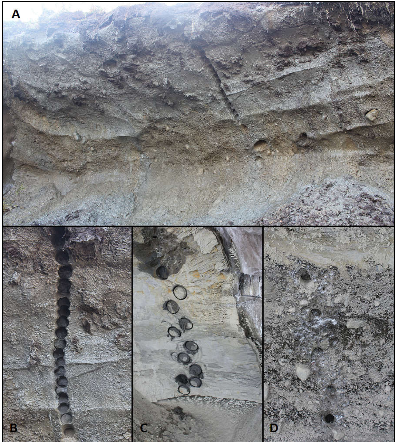
Figure 20. Sample extraction from the headwall at Two Moose Lake during August 2013 (A & B) and April 2014 (C & D). A) Headwall showing the location of sample extraction using a Hilti power drill with a 8cm diameter corer with diamond-embedded cutters (0.25-1.9m). Samples below 1.9m were removed using an ice pick (not visible). Sample extraction using a Hilti power drill from B) 0.25-1.9m showing the slight overlapping of samples during August 2013; C) 1.75-3.15m during April 2014 and; D) 3.15-4.35m (lowest exposed unit) from April 2014.
