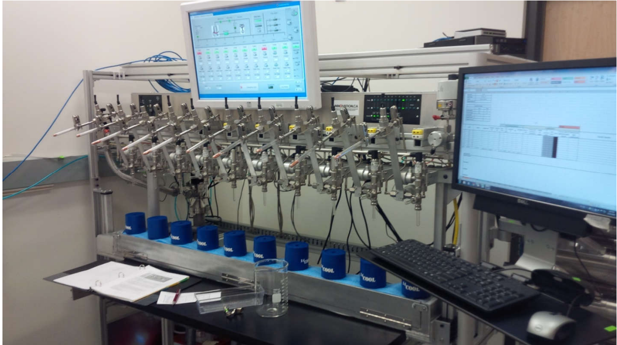
Figure 23. Automated Graphitization line at the Radiocarbon Lab (A.E. Lalonde AMS Laboratory, University of Ottawa) used in the reduction of CO 2 to graphite for subsequent analysis on AMS.
