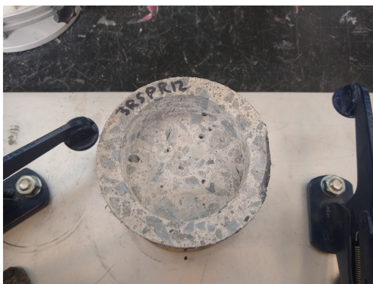
Figure 4.5: Powder extracted from a specimen up to 13 mm.
