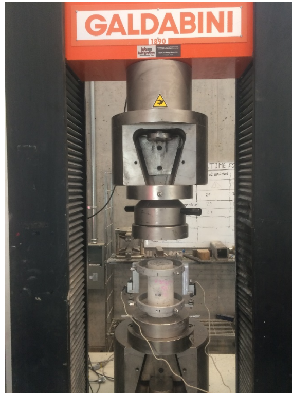
Figure 4.4: SDT test setup for cylindrical concrete specimens.
