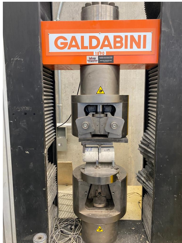
Figure 4.3: Shear setup for cylindrical concrete specimens [5].
