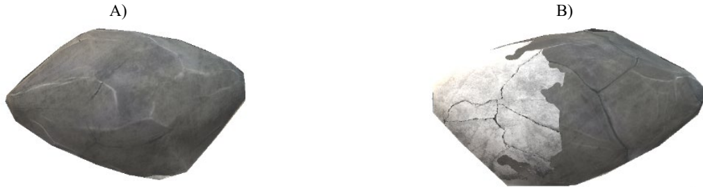
Figure 7.1: A model showing A) coarse virgin aggregate and B) coarse RCA (RM and OVA).
