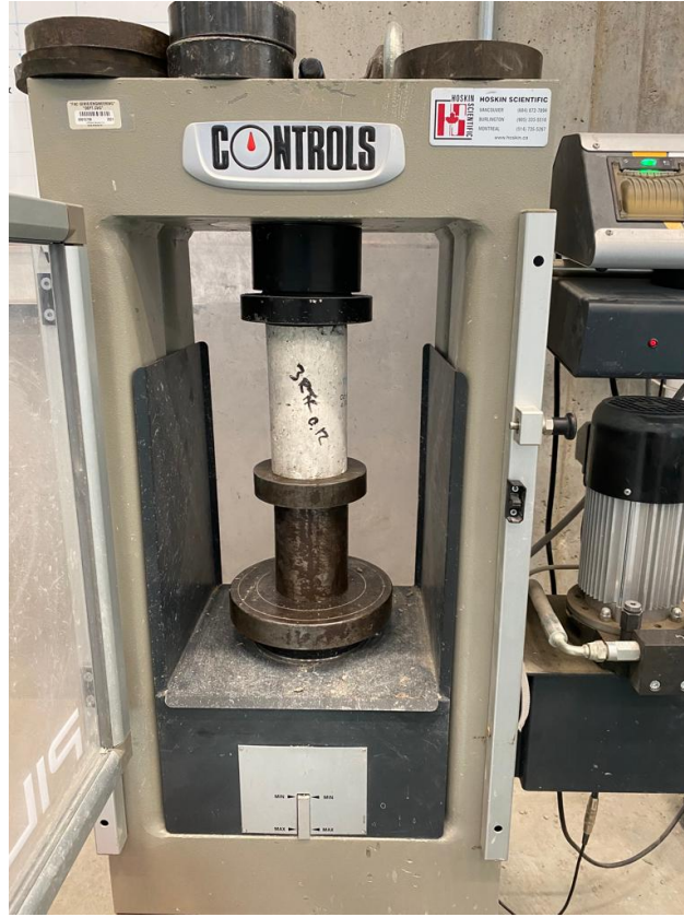
Figure 4.2: compressive strength test setup for cylindrical concrete specimens.
