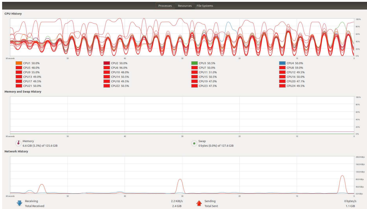
Figure 3.17: CPU usage when running the real-time Python application using multiple processes and threads.
