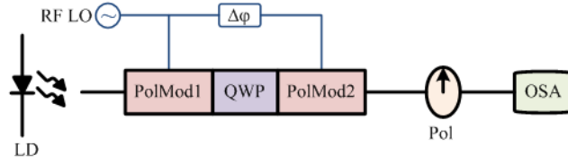
Fig. 1. Schematic diagram of the proposed frequency up-converter. LD: laser diode; PolMod1: polarization modulator 1; QWP: quarter wave plate; PolMod2: polarization modulator 2; Pol: polarizer; OSA: optical spectrum analyzer. RF LO: radio frequency local oscillator.
