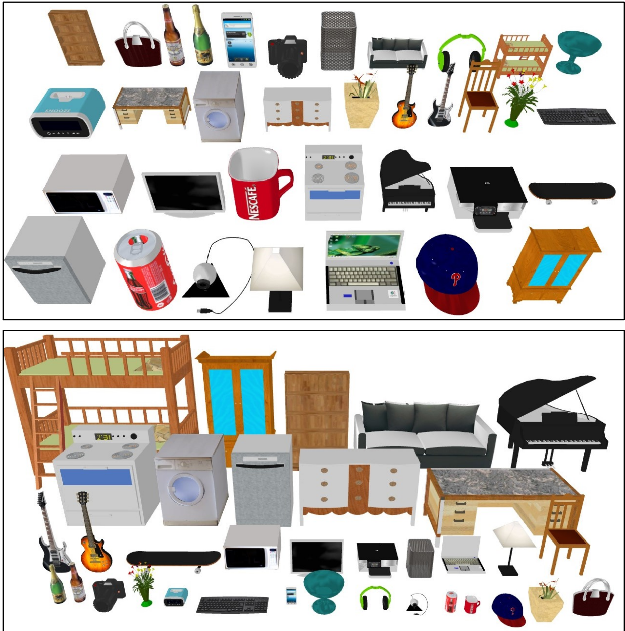
Figure 6.4. (a) Offline-learning to assign absolute sizes to 3D models. The upper row demonstrates a collection of 3D models in their default sizes; Same models are shown in the lower row after being automatically scaled using the offline-learning. Size distributions of objects are learned from various retail store websites such as Walmart, IKEA, etc.
