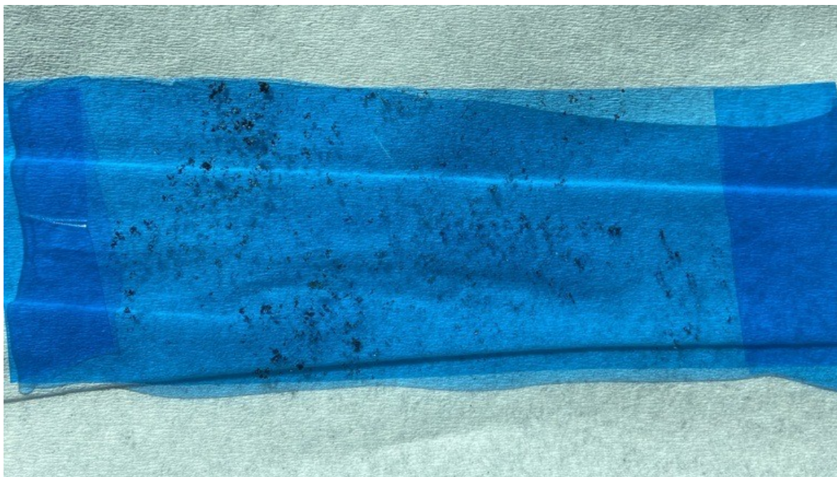
Figure 27: Image of the tape exfoliation, corresponding to step D of Figure 26
