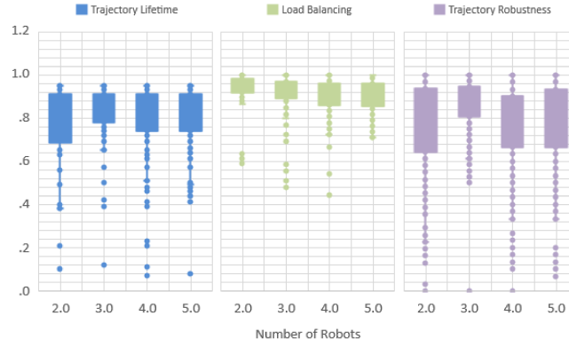
Fig. 5. Normalized values for objective functions (2), (3), and (4) using the Pareto set from the generated reference set for the representative instance file
