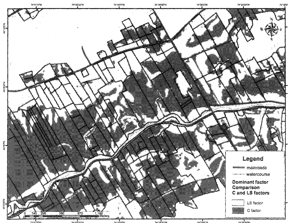
Fig. 93. Most dominant factor effecting erosion when comparing the LS and C factors for a portion of South Nation watershed, under 25% LS field boundary connectivity, with 2001 conservation tillage practices.
