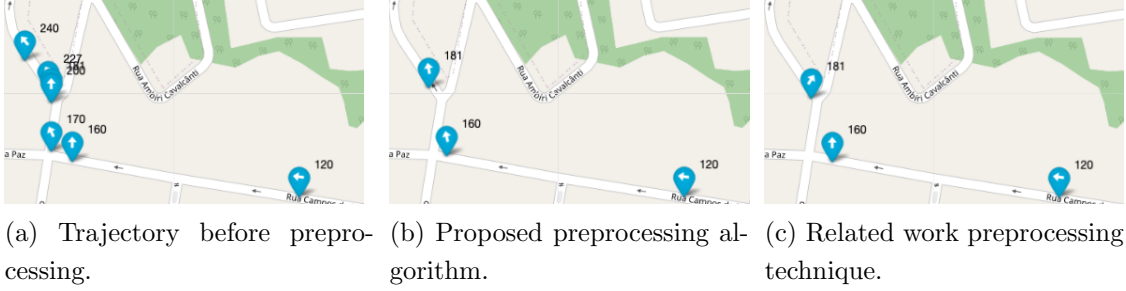
Figure 5.3: Comparison of the proposed preprocessing technique and relate work.
