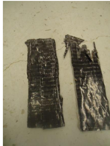
(b) Failure in the gripping area
