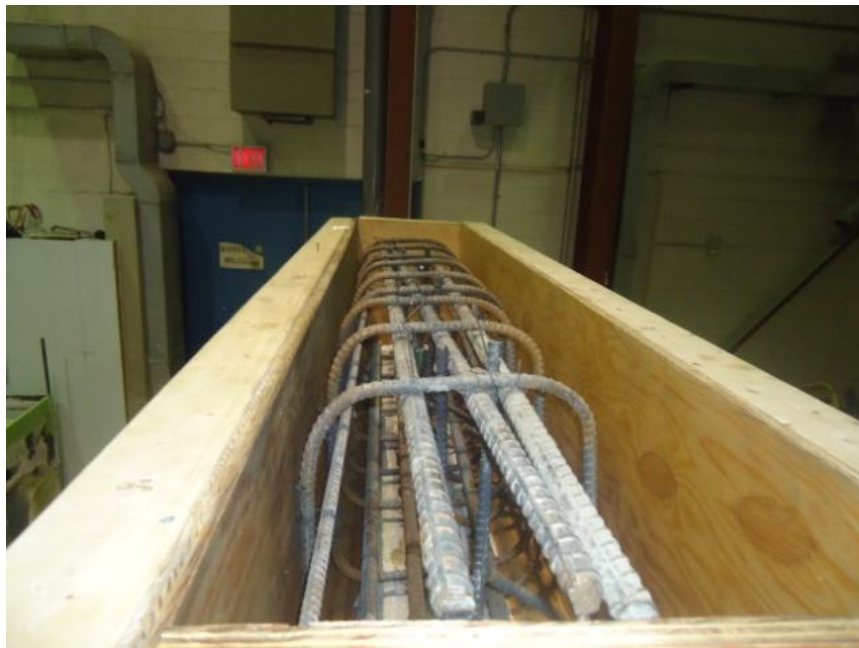
Figure 4.5: Reinforcement cage in top beam for PRM wall
