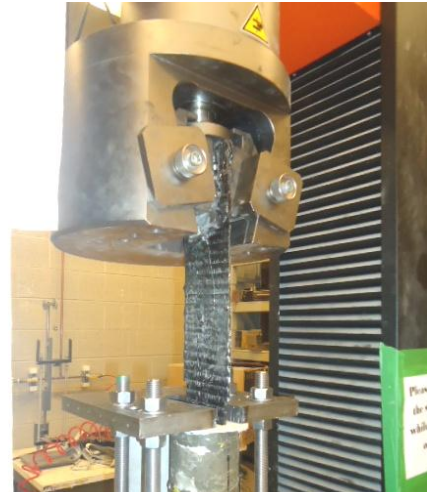
Figure 3.2: Test of FRP laminates inserted in concrete cylinders
