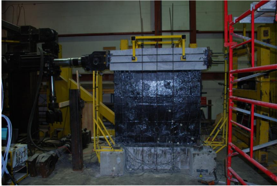
Figure 4.33: PRM wall prior to testing
