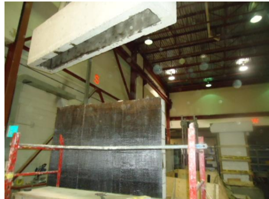
Figure 4.12: The placement of precast top beam on the wall
