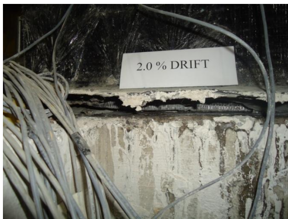
(c) FRP Separation at 2.0% drift
