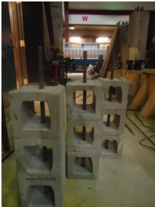
(a) Masonry blocks with #20M rebar
