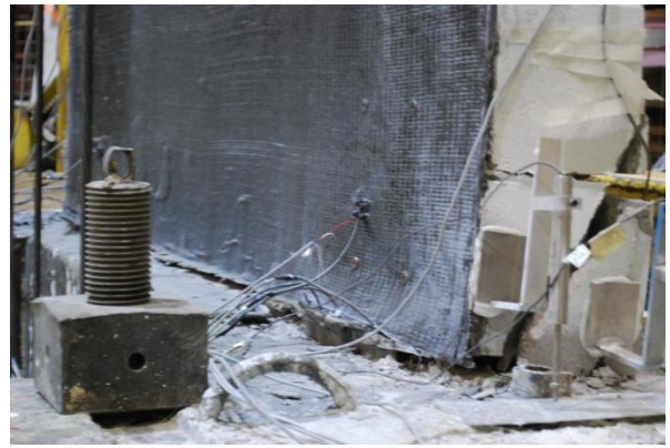
(d) Extension in tension and buckling in compression of steel sheet anchors; 1.5% drift
