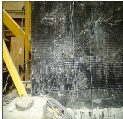
Figure 3.1: Application of FRP fan type anchors
