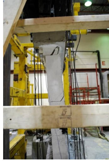
(b) Twisting of the wall at 1.5% drift
