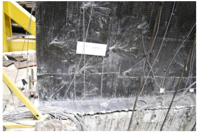
(b) Wall rocking at 1.75% drift
