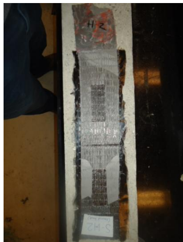
Specimen after bond failure
