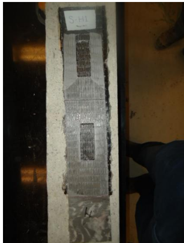
Specimen after bond failure
