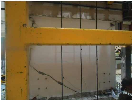
(c) Unretrofitted side of wall at 0.5% drift
