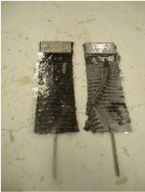
(a) Curved wire sandwiched in CFRP sheets
