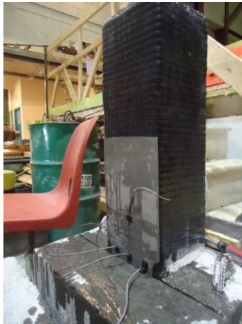
(a) Placement of anchor
