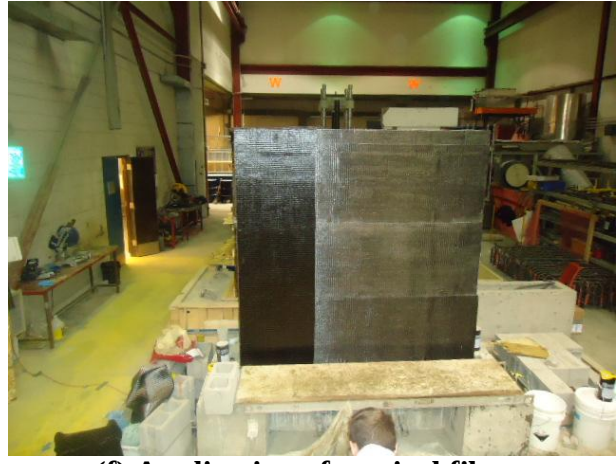
(f) Application of vertical fibres
