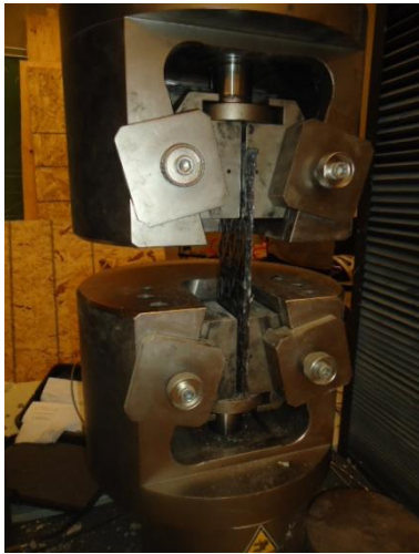
(a) Test of a FRP-steel mesh composite anchor
