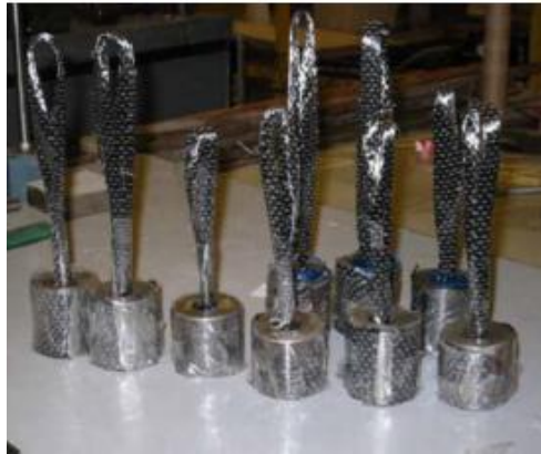
Figure 2.4: FRP anchors placed in a steel barrels as part of a test setup ( Adapted from Ozbakkaloglu et al. 2009)
