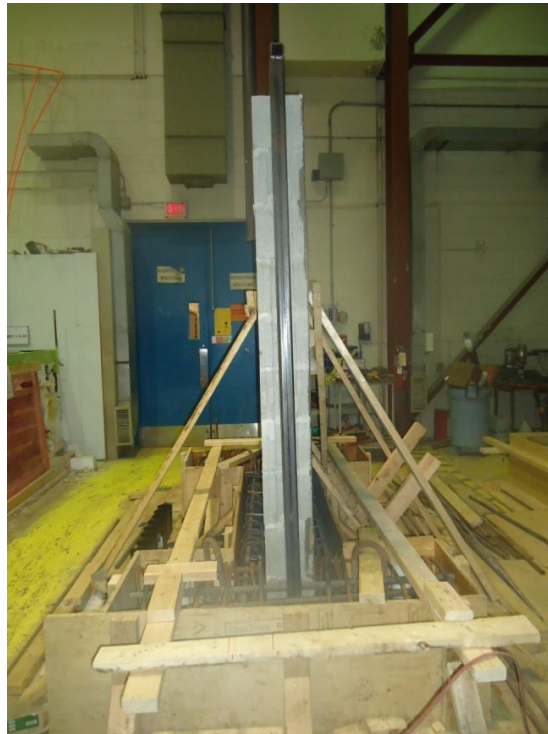
Figure 4.2: Integration of wall with reinforced concrete foundation
