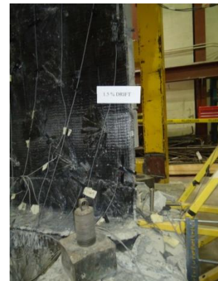
(f) Performance of anchors at 1.5% drift
