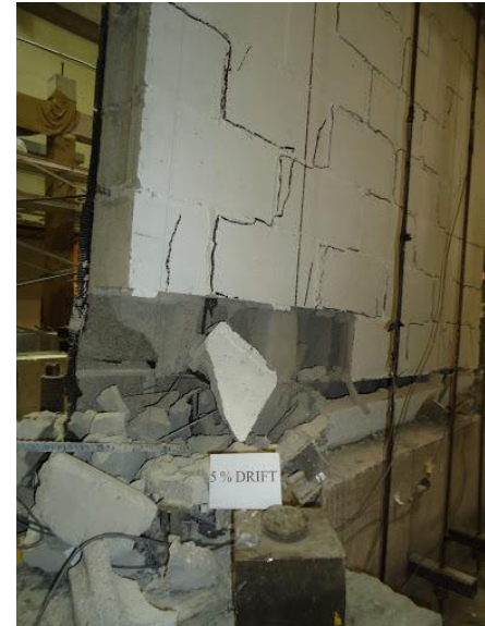
(b) Crushing of east end at 5% drift
