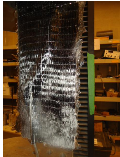
(b) Bond failure surrounding the wire
