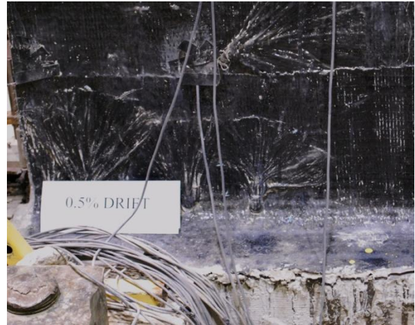
(b) FRP fan anchors at 0.5% drift
