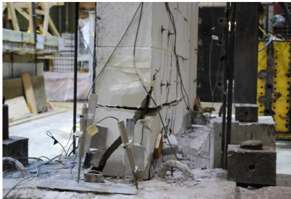
(c) Twisting of wall at the east corner; 1.5% drift
