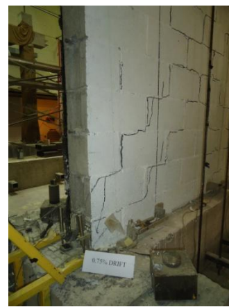
(f) Corner crushing, east end, 0.75% drift
