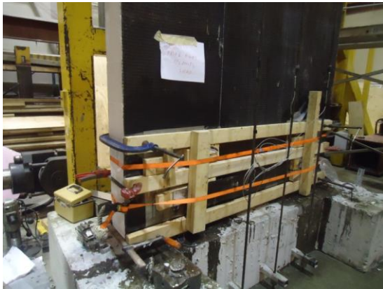
(a) Clamping of anchors
