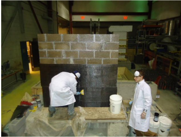
(e) Application of horizontal fibres
