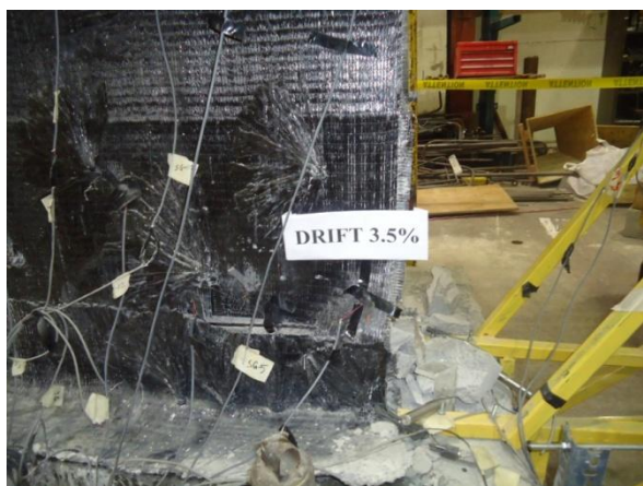
(e) FRP delamination at 3.5% drift
