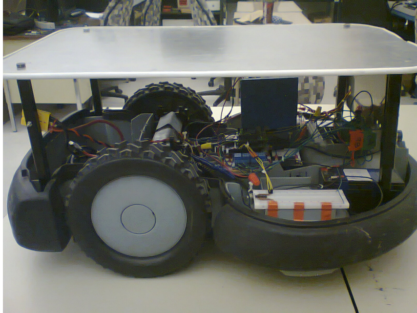
Figure 4.3: Platform with Aluminium roof.
