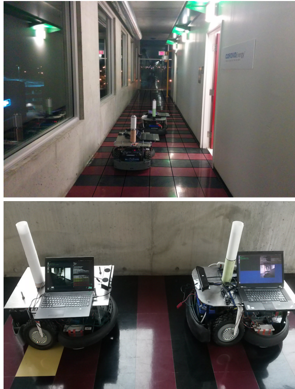
Figure 4.23: Experimental setup for evaluation of multirobot localization.
