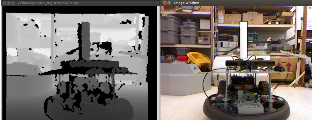
Figure 4.21: Depth Image (Left) and RGB Image (Right) from Kinect with a joystick-controlled line cursor (Green).
