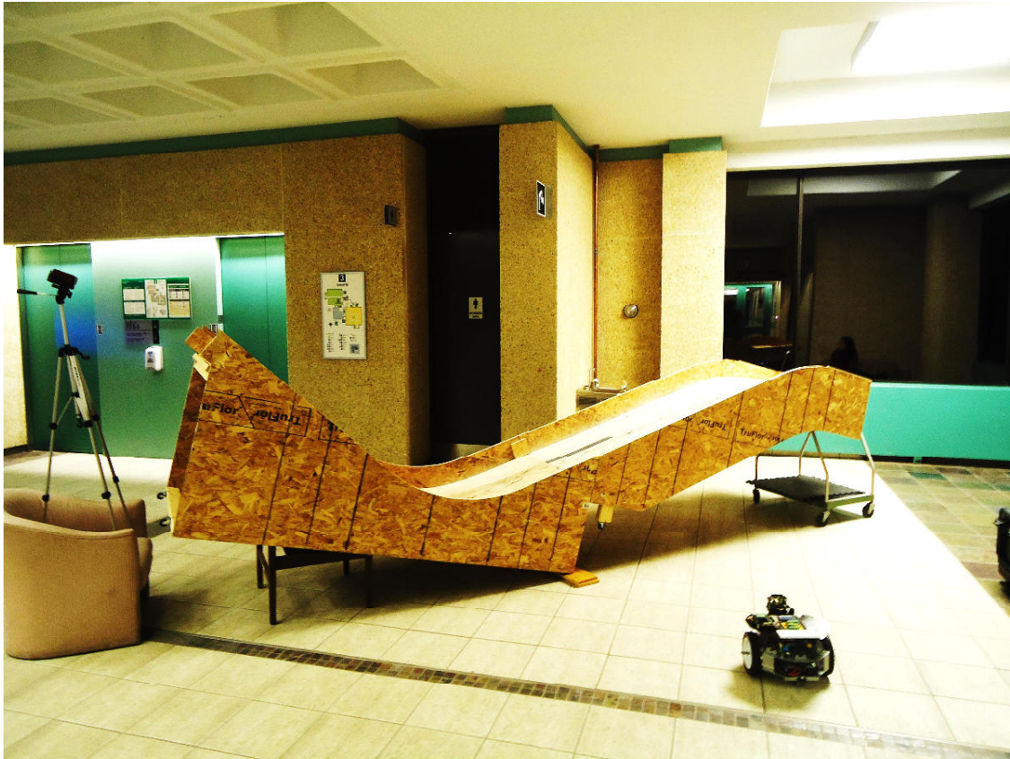
Figure 3-2: A ramp setup that provides 47^{\circ} downhill ramp with 13^{\circ} uphill ramp.
