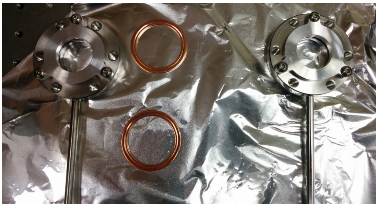
Figure 5.4: Image of unmounted differentially pumped IR windows with KBr crystals.
