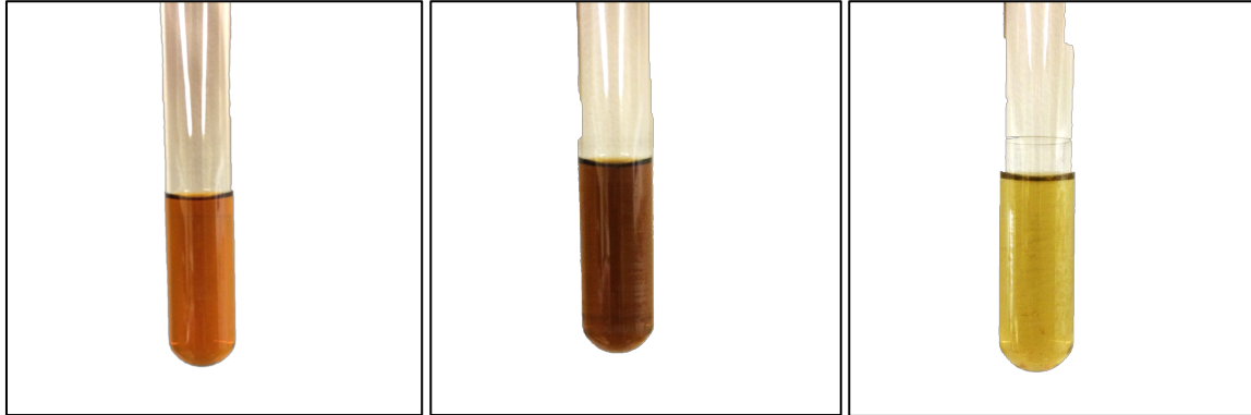
Figure 5-1 Progression of colour change resulting from to G. metallireducens growth in ATCC 1768 media. From left to right, appearance of hungate tube upon inoculation, after 72 h of growth, after 160 h of growth.
