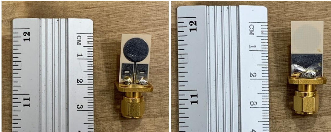
Figure 5-5 CBCPW MMW antenna prototype for U_{\text{band}} (a) top view, and (b) bottom view
