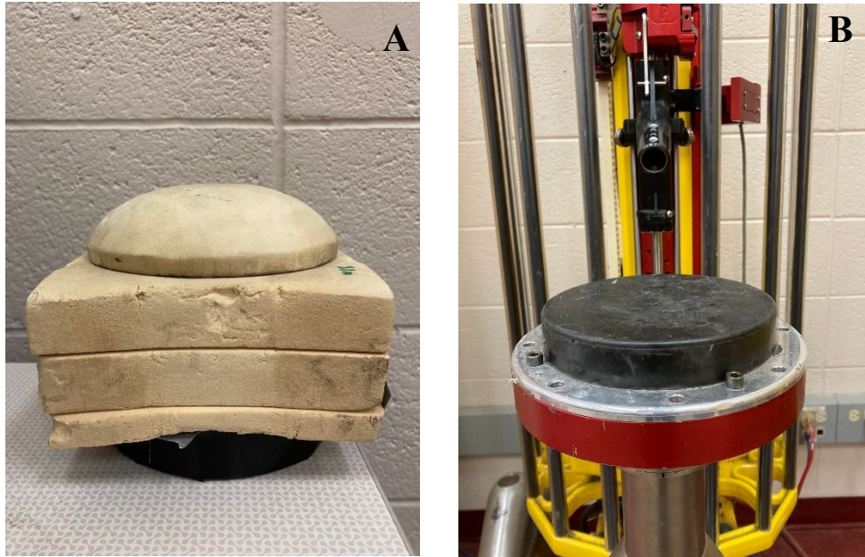
Figure 5. Anvils used to represent different contact surfaces for the body tracking reconstruction method: (A) shoulder & elbow, (B) boards & ice
