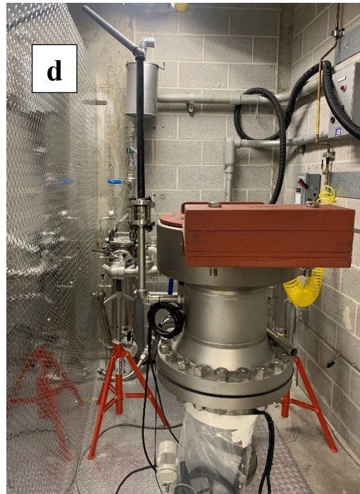
Fig. A - 2. This image outlines the different parts of the fluidization system. a) fluidization column, b) bottom manway, c) the knife gate valve used as a distributor plate, and d) top manway
