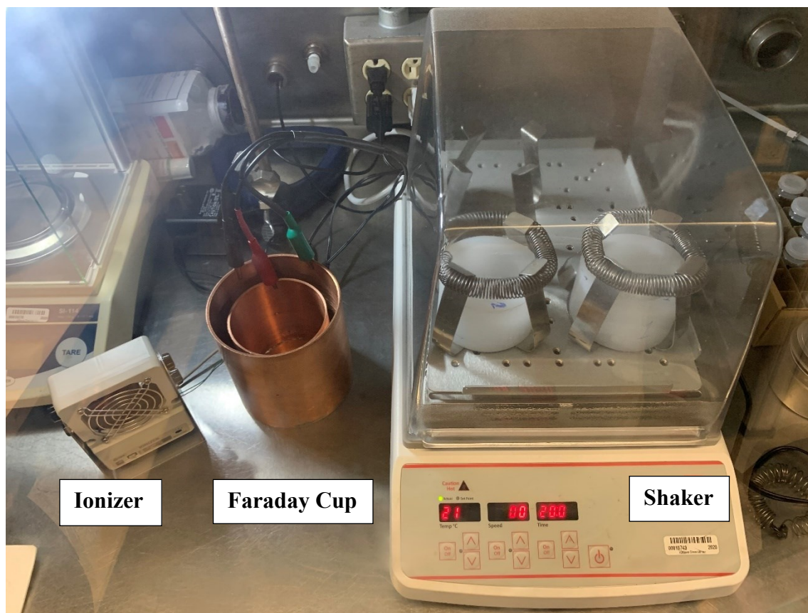
Fig. A - 4. Shake test apparatus in a glove box filled with nitrogen
