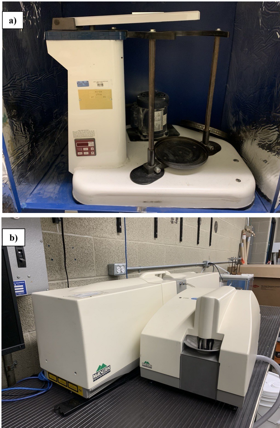
Fig. A - 7. Particle size distribution measurement techniques. a) Sieve test, b) Malvern Mastersizer 2000.
