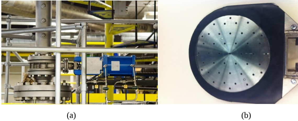
Figure C.3: Pictures showing (a) the knife gate valve; (b) the modified blade of knife gate valve to serve as the perforated plate.
