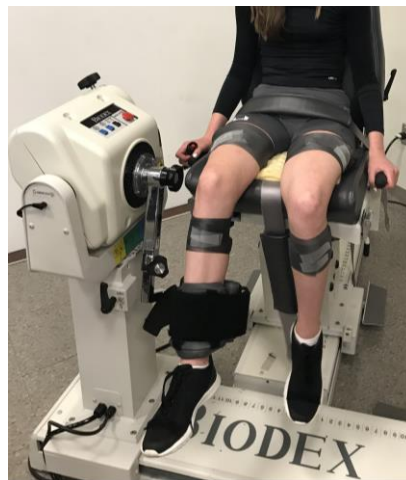
Figure 1: Maximum voluntary isometric contraction performed on a biodex isokinetic dynamometer. Participants were seated with their knee held at 60 degrees.
