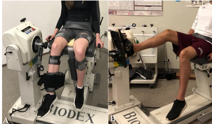
Figure 5.1: Participants position during knee extension (A) and ankle plantarflexion (B) isometric test
