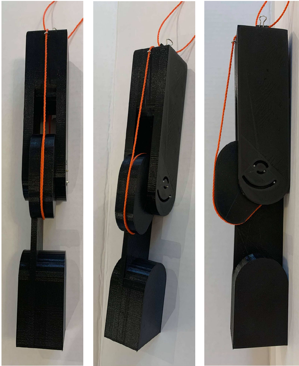
Figure 5.2. Experimental prototype of the joint with no offset. The femoral and tibial components are constructed out of PLA with steel pins. The cable (bright orange) is made of polypropylene mason twine and is fed through eyelets on the anterior and posterior ends of the femoral component.
