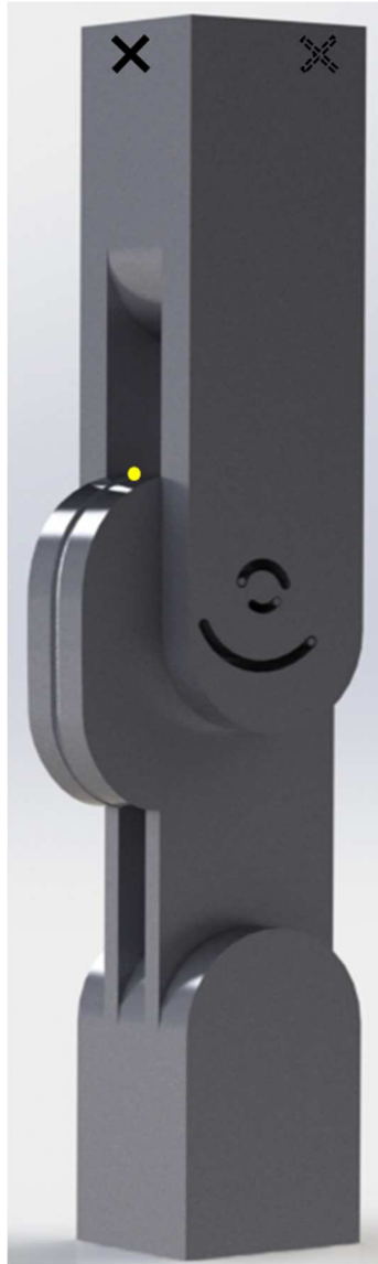
Figure 3.11. SolidWorks assembly of joint without offset. Cable and bushings not depicted. Location of pretensioner pulleys indicated by black 'x' markers and location of pin indicated by a yellow point.
