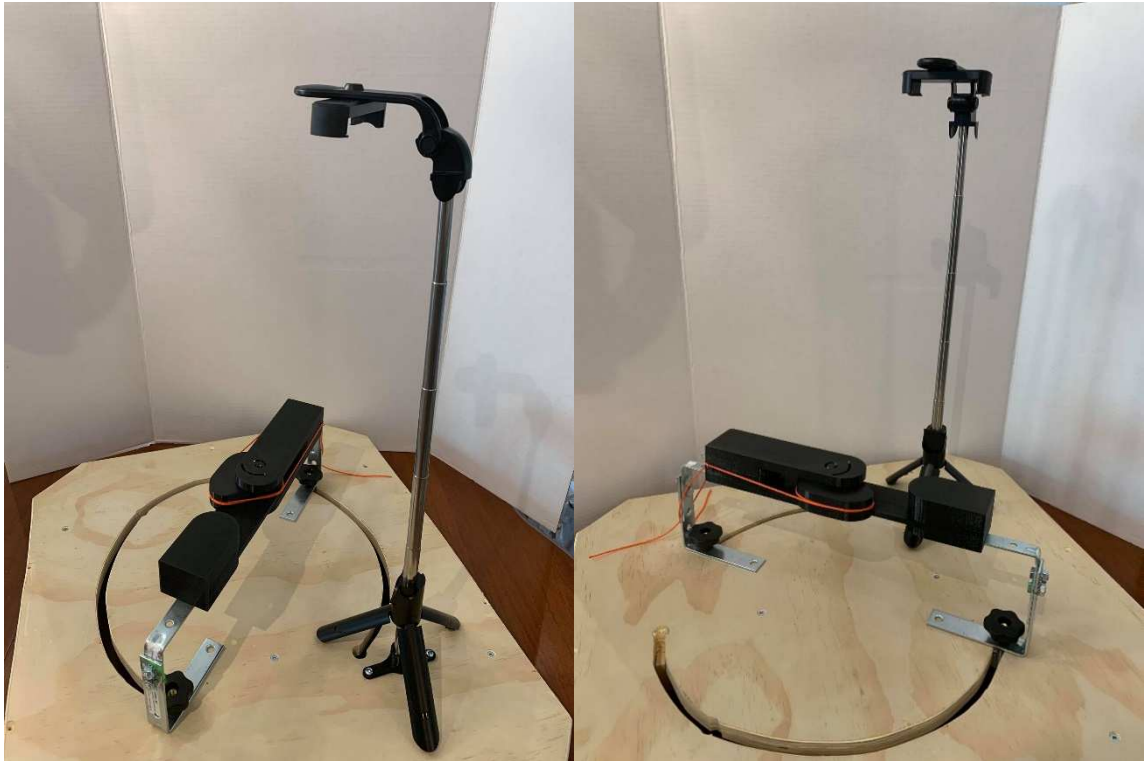
Figure 5.4. Testing rig 1. Prototypes are fixed to a board with two curved tracks by adjustable U-shaped supports. A tripod is fixed to the board to take photos of the prototypes at prescribed intervals of 15^\circ .
