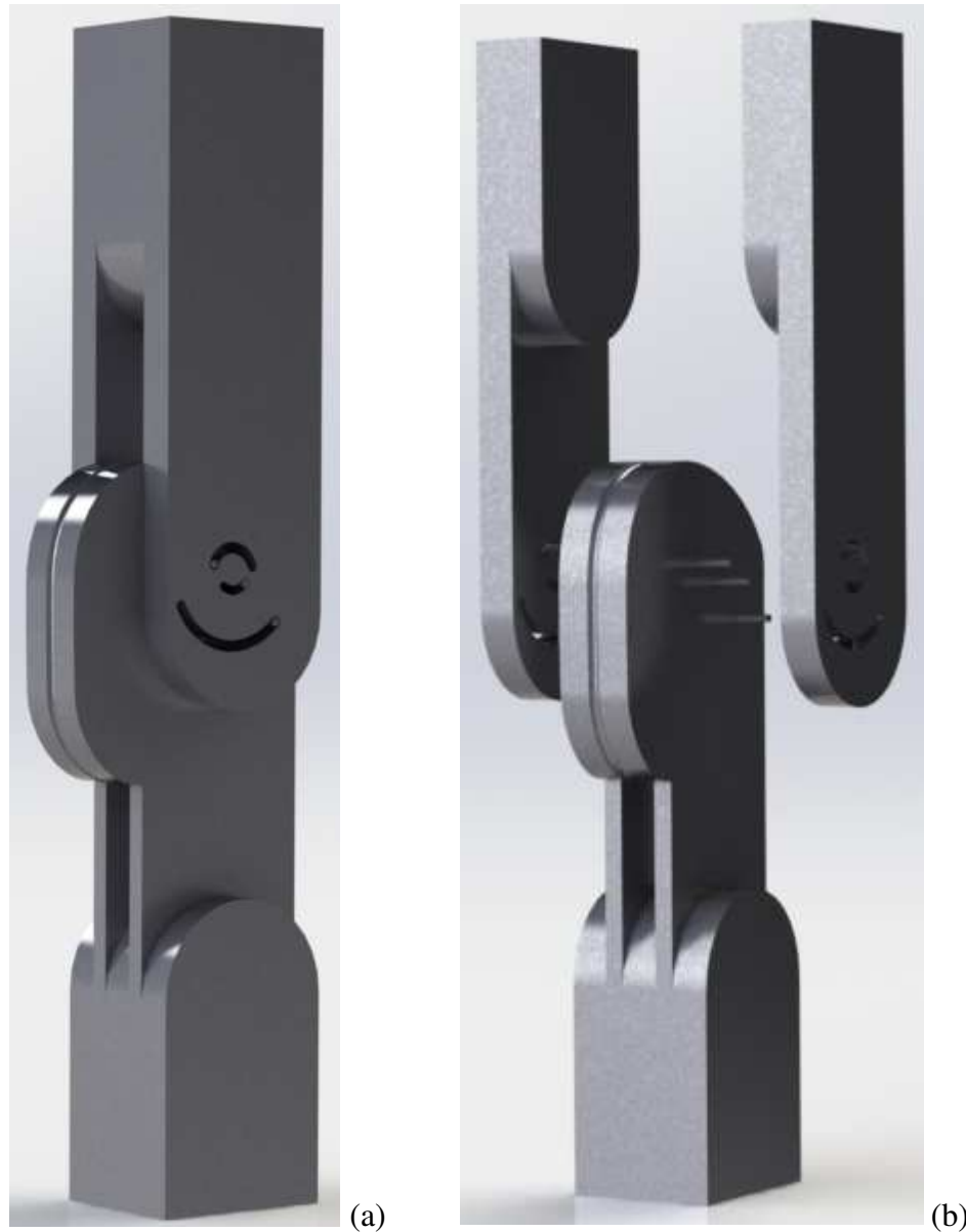
Figure 3.9. SolidWorks assemblies of the joint design concept. A tibial component with pins is shown between two femoral components that have slots. (a) Intact assembly, (b) exploded view.
