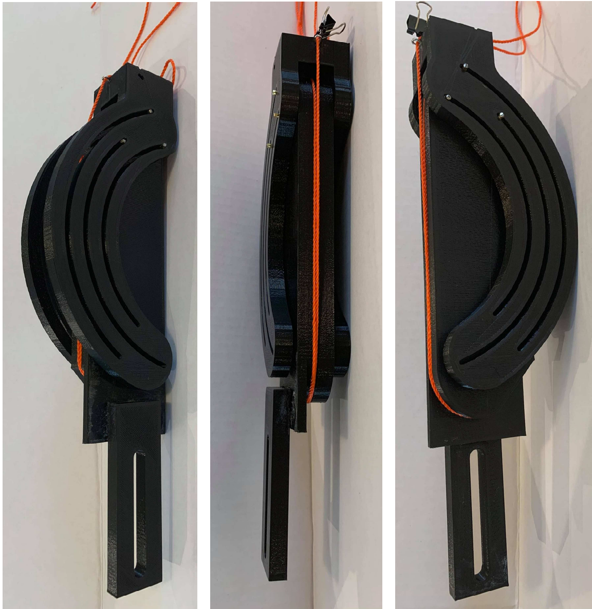
Figure 5.3. Experimental prototype of the joint with offset. An extension with a slot is added to the tibial component to allow for use with the testing rig.
