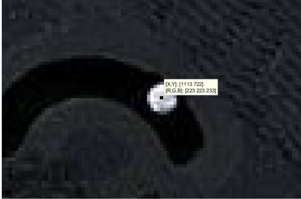
Figure 6.4. Manual identification of the center of a pin using data cursor in MATLAB.
