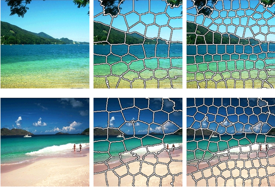
Figure 4.1: SLICO segmentation results: the left are original images, the middle column shows segmented results with N_{SP} = 43 , while the right for N_{SP} = 100
