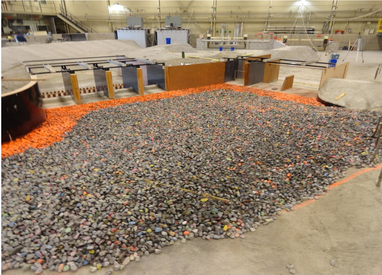
Figure 43: Finished flow structures with riprap placed directly upstream (NRC, 2016)
