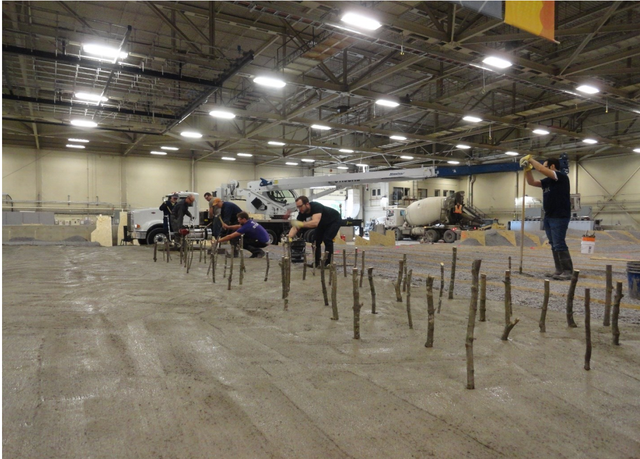
Figure 40: Grout finishing and installation of scaled trees (NRC, 2016)
