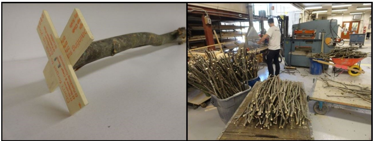
Figure 4: Root Wad attached to LWD (left), debris fabrication at NRC facilities (right)
