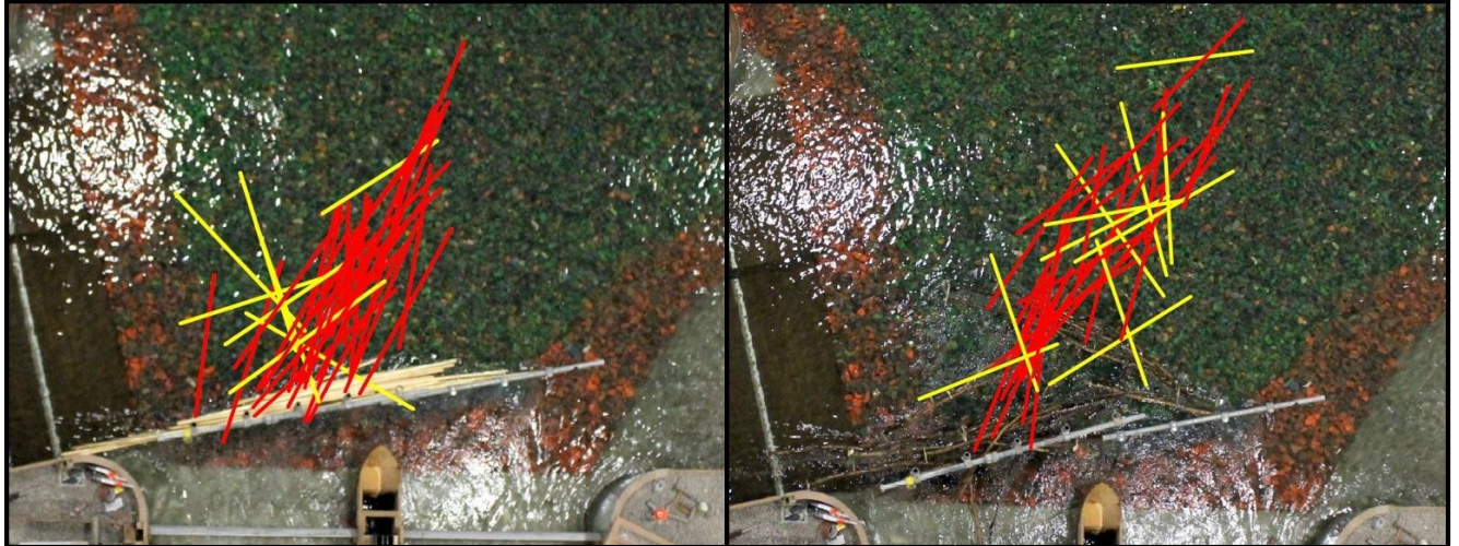
Figure 7: MD (left) and RDR (right) angle of arrival with pieces greater than one standard of deviation from the mean highlighted in yellow
