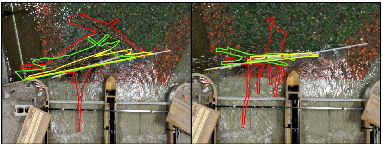
Figure 8: Outline of single debris test dam (left) and a 10-piece dam (right) for all debris types. MD yellow, RDN green and RDR red.
