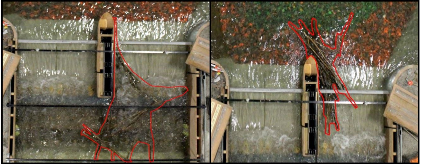
Figure 5: 17 piece dam jammed due to root wad (left) 38 dam jammed due to debris roughness (right) with no debris rack in place
