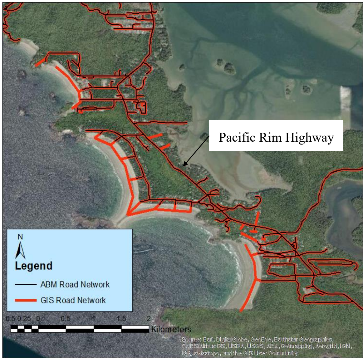
Figure 20: The black roads were used in the ABM as pathways for agents to traverse on. The ABM road network was then replicated into the GIS model, but additional roads were required due to nature of the agent behaviour. The road network used in GIS model is shown in red.
